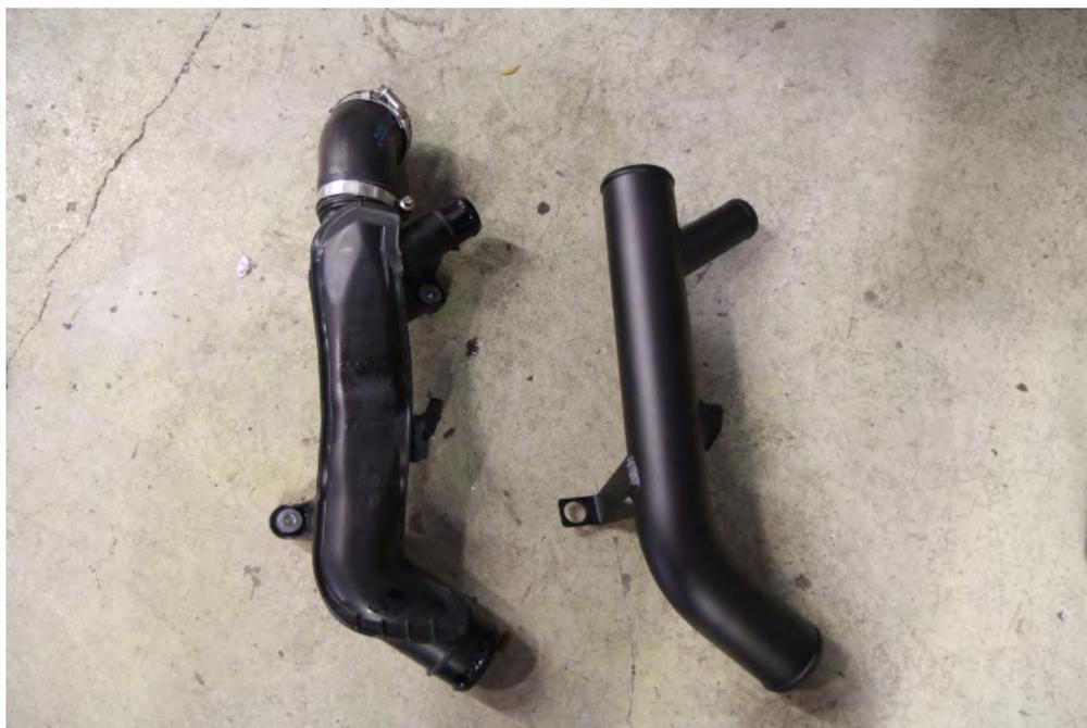
Step 8: Transfer the bottom mounting bracket hardware (rubber bushing with metal sleeve) to the new throttle pipe. Using a Philips screwdriver, remove the MAP sensor off the old pipe. Reattach to the new pipe using an 8mm socket and the supplied bolts.
