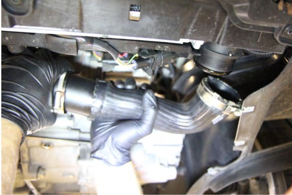
Step 15: Take the pipe cap and install it with the supplied clamp over the exposed end of the pipe. Reinstall your engine cover with airbox. You are done!
