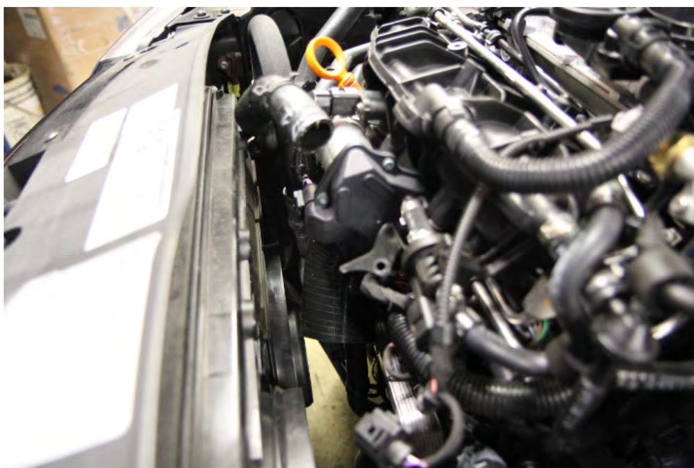
Step 11: Place the second hose clamp loosely over the top of the throttle pipe and feed the pipe up from the bottom inserting it into the upper silicon hose. Tighten the hose clamp over the silicon and pipe joining the throttle pipe to the throttle body.
