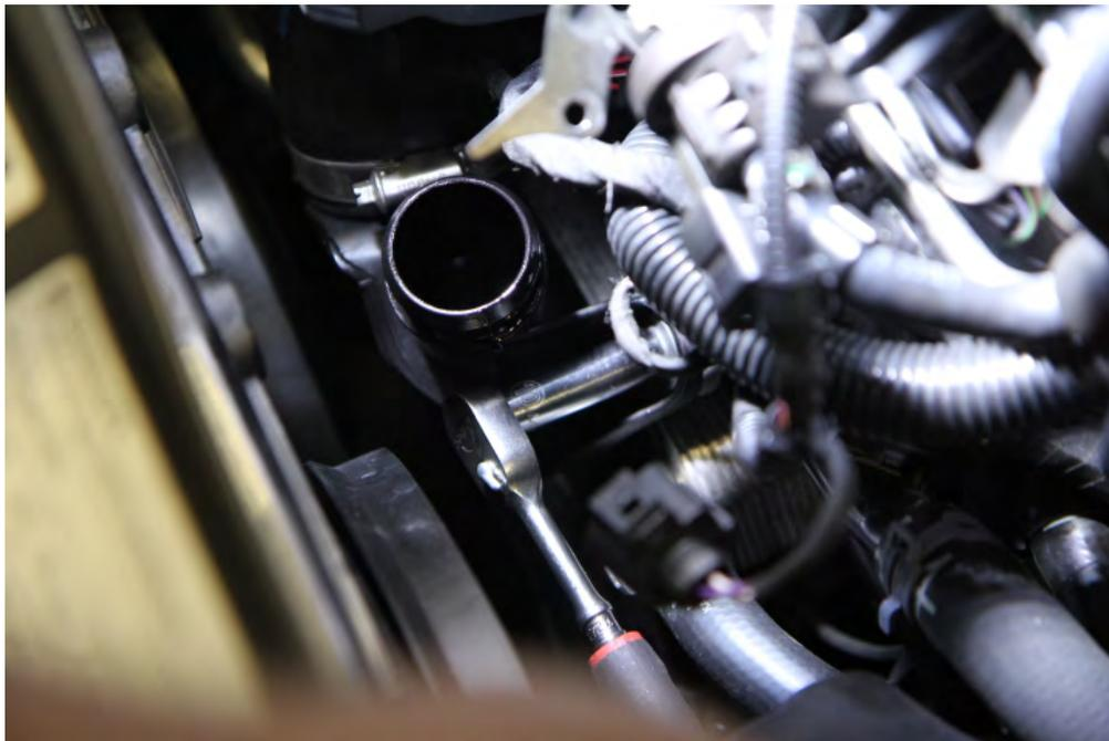
Step 5: With the car up on a hoist or on jackstands. Use a T30 Torx bit to remove the bolt holding the bottom bracket of the throttle pipe to the engine.
