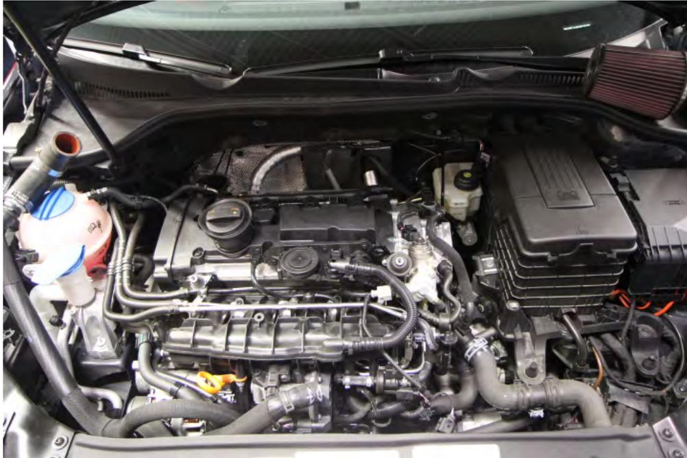
Step 2: Using a ratchet with an 8mm socket, loosen the 2 hose clamps at the top of the throttle pipe connecting it to the throttle body. (Golf R OEM pipe seen here).
