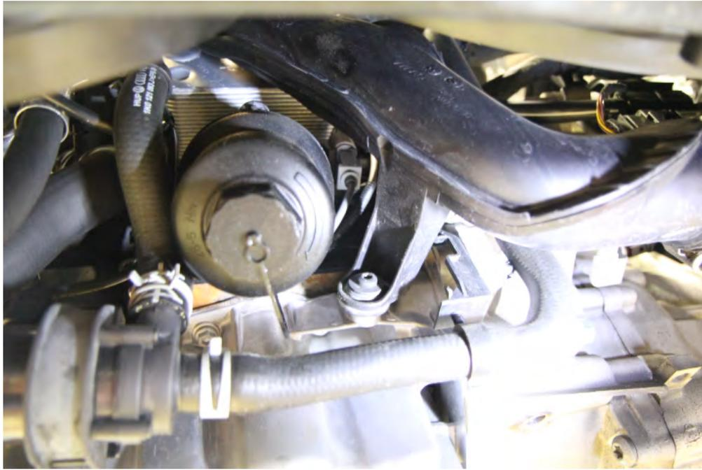
Step 6: Using a flathead screwdriver or 8mm socket, loosen the 2 hose clamps holding the rubber hose to the bottom of the throttle pipe and the intercooler. Pull the hose free.
