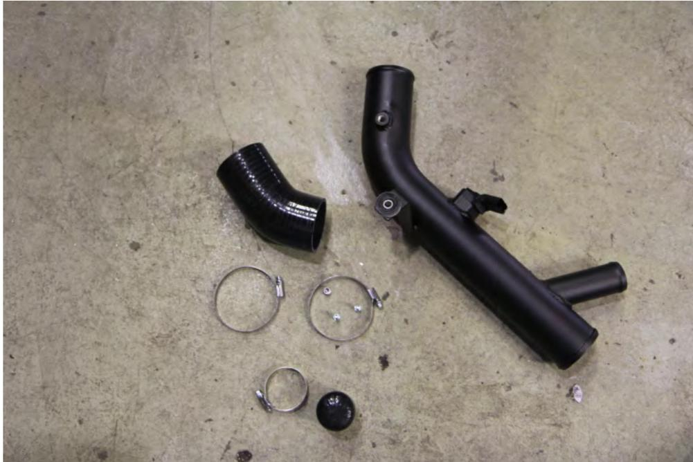
Included in the kit: Intake pipe, 2 hose clamps, 2 M8 bolts, 1 water/meth bung plug, 1 silicon pipe connector (if installing on GTI/Jetta, you will receive a 1 hose clamp, 1 silicon pipe cap).
