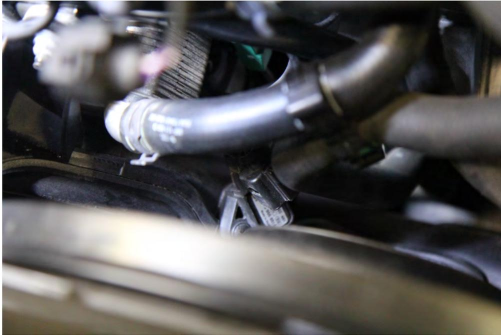
Step 4: Using a ratchet with a 10mm socket, undo the bolt holding the top bracket of the throttle pipe to the engine.
