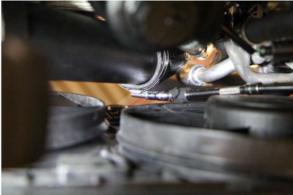
Step 12: Using the T30 Torx bit, reattach the bottom bracket of the throttle pipe to the engine.
