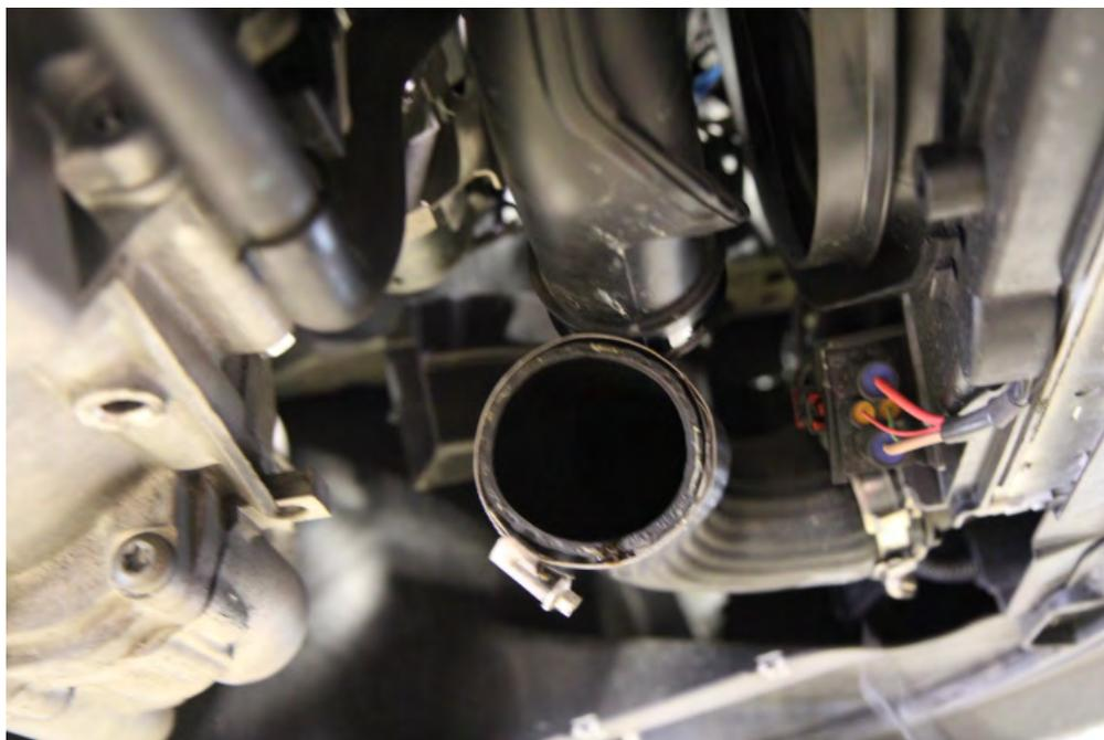
Step 7: Wiggle the entire throttle pipe assembly down and out of the car.
