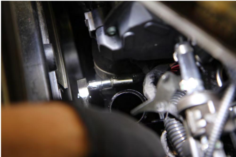
Step 3: Pull the connector off of the the MAP sensor located halfway down the stock throttle pipe.
