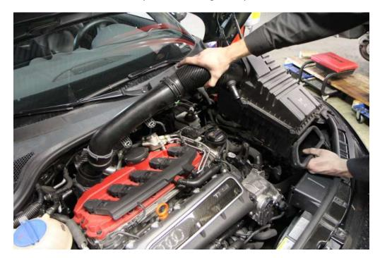
**Step 9:** Pull the 2 rubber mounting grommets free of the OEM airbox and reinstall in the supplied CTS airbox. Place the CTS airbox into the engine bay and press down on the 2 mounting points to seat the box.
