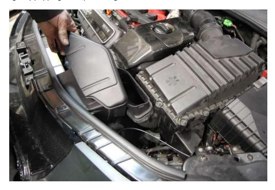
**Step 2:** Use your flat head screwdriver to pop the 2 clips on the left and right side holding the air inlet to the front assembly. Pull free.
