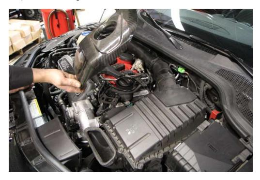
**Step 4:** Use your pipe clamp removal tool to release the rubber diverter valve outlet hose from the OEM pipe. Pull the rubber hose free.
