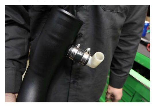
**Step 12:** Install the pipe into the car. Seat the left side of the CTS pipe into the OEM silicone. Reinstall the diverter valve outlet hose to the 90 degree elbow.
