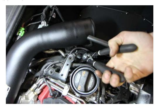
**Step 14:** Use your 5mm allen socket to install the M6x16 bolt securing the pipe to the engine.
