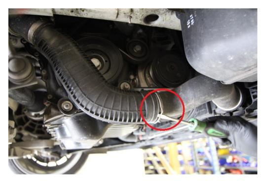
**Step 4**: Use the T30 torx bit to remove the 2 bolts holding the plastic pipe to the engine.
