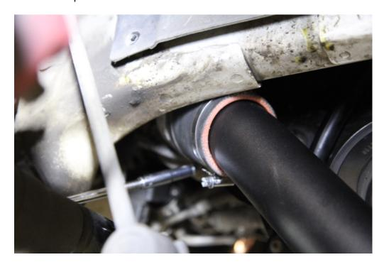
**Step 11**: Reinstall the 2 T30 torx bolts holding the pipe to the engine.
