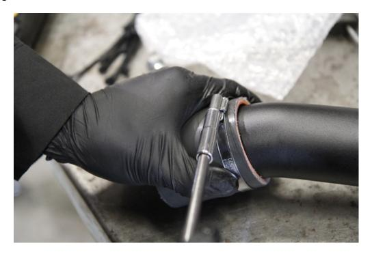
**Step 10**: Manouver the outlet pipe into position sliding the silicon over the turbo connector. Tighten the hose clamps over the silicon.
