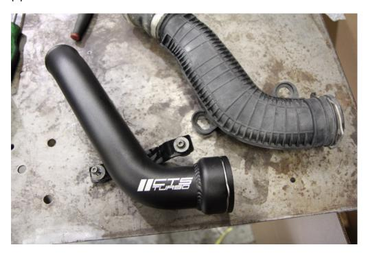
**Step 9**: Slip the 2 hose clamps onto the silicon connector then slip the silicon connector onto the discharge pipe. Loosly tighten both of the clamps on either end of the silicon to avoid slipping.
