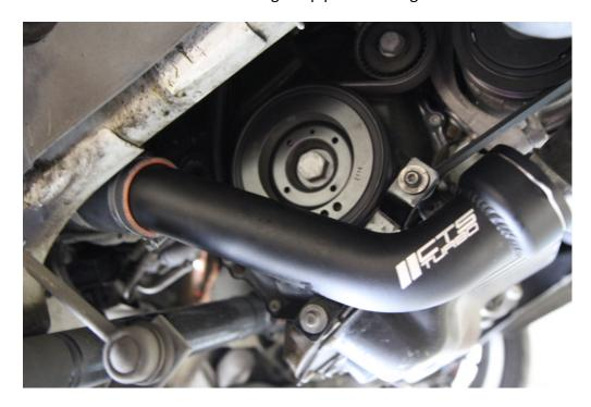
**Step 12**: Reinstall the rubber intercooler hose with the retaining clip. Reinstall the inner fender liner and engine pan. You are done!
