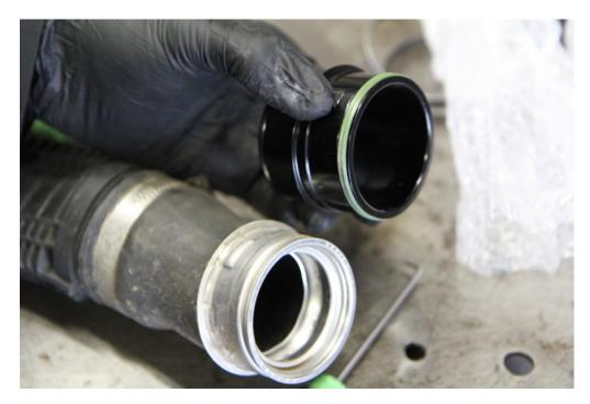
**Step 7**: Reinstall the retaining ring onto the turbo, then snap the new billet outlet into place.
