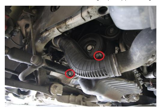
**Step 5**: Using the screwdriver, pop the retaining ring off of the upper pipe joint then pull the plastic discharge pipe off of the vehicle.
