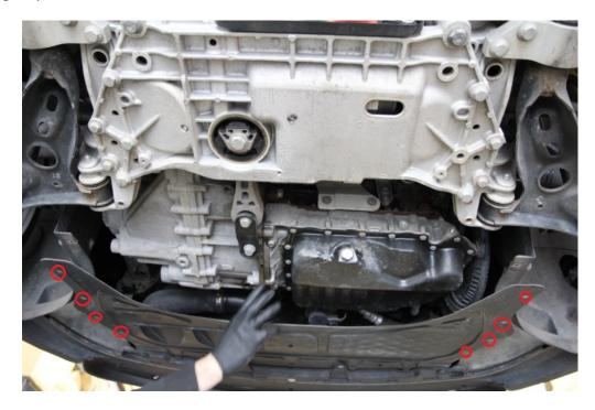
**Step 2**: Remove the 7 T25 torx bolts holding the passenger side lower inner fender liner to the car. Note that 2 of the torx bolts are under the front bumper cap. Pull the liner free.
