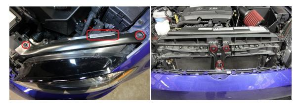
Step 2: Remove headlight washer line (squeeze the blue tabs), drain washer fluid and unclip the hose. Remove the hose from the retaining clips along the top of bumper.
