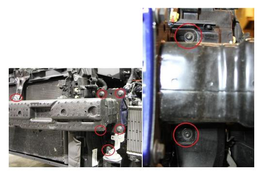
Step 6: Remove plastic air deflectors and unclip the factory snap-connectors for the intercooler. Use grease or WD40 to help with removal.
