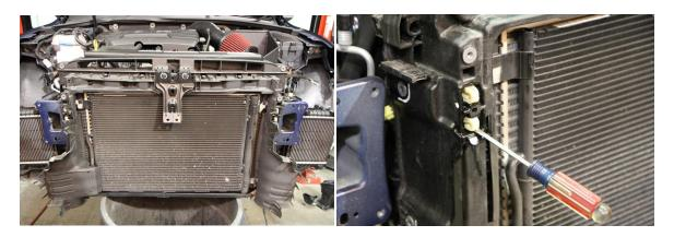
Step 7: Remove the radiator support and a/c condenser. Unclip the factory FMIC from the radiator and remove.
