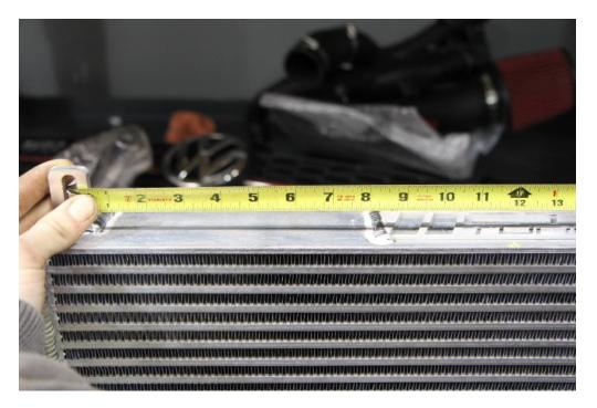
**Step 8:** On the crashbar, mark 11.75" to the left and right of the center line. Mark mounting holes, try to align mounting holes in the middle of the crash bar.
