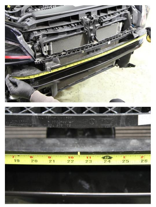
**Step 7:** Measure 10.75" from the middle of the right hole on intercooler mounting bracket and mark the center line.
