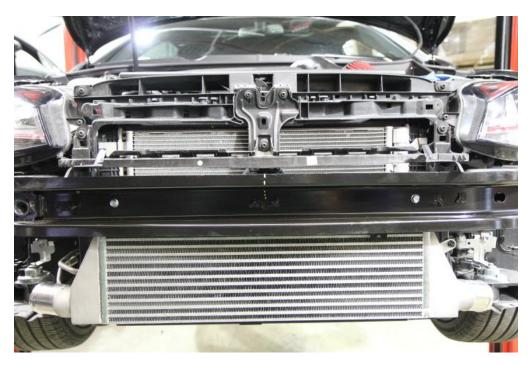
**Step 10**: Remove the temperature sensor from the mounting bracket, install the intercooler using supplied M8 bolts, and reinstall the temperature sensor as shown.
