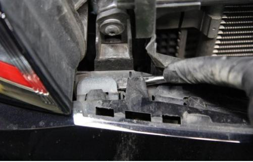
**Step 6:** Remove the foam crashbar. Measure 22.5" from the right side of the car and mark the center line.
