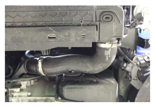
**Step 15:** Install CTS Turbo hoses, do not overtighten clamps.
