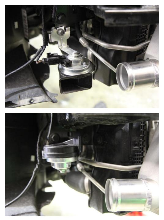
**Step 12: OPTIONAL**, this step applies only to cars with SAI system - remove the mounting bolt for SAI pump, loosen the second mounting bolt on the back. Install supplied bracket to move pump out of the way.
