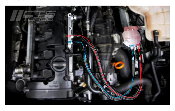
Step 5: Install the PCV Plug into the intake port shown. Lock in place by twisting forward.
