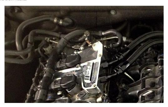
Step 3: Using the included bracket, mount the catch can to the car. See photos for reference.
