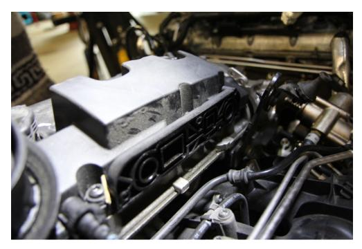
Step 2: Remove the OEM gasket from the factory breather plate and insert into the replacement breather plate. Reinstall the breather plate using the OEM T25 torx screws. For TSI, use supplied bolts. Reattach breather hose as shown.
