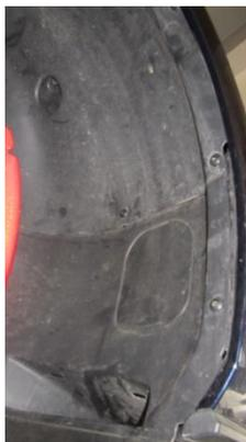
6. Remove the two M10 nuts that hold the slam panel to the crash bar .
