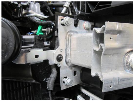
21. Using your T27 torx driver, remove the fastener next to the 17mm bolts.
