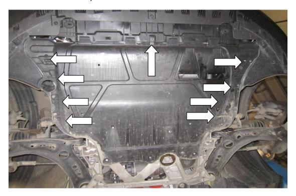
6. Using your T25 torx drive, remove the three fasteners at the front of the bumper underside. While in this position undo the boost hoses with your hose clamp drive.
