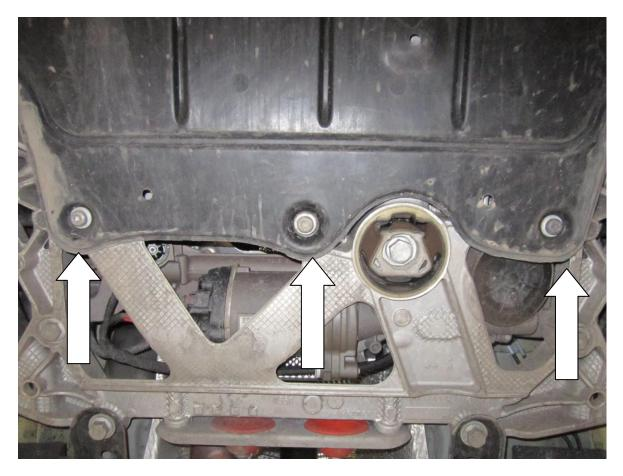
5. Using your T20 torx drive remove the fasteners that hold the sides of the undertray to the lower of the arch liners. Please also remove the T20 fastener in the middle at the front of the undertray. There are nine fasteners in total.
