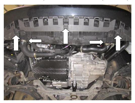
7. Using your T20 torx drive remove the fasteners at the front of your inner arch liners; there are six in total on each inner arch .
