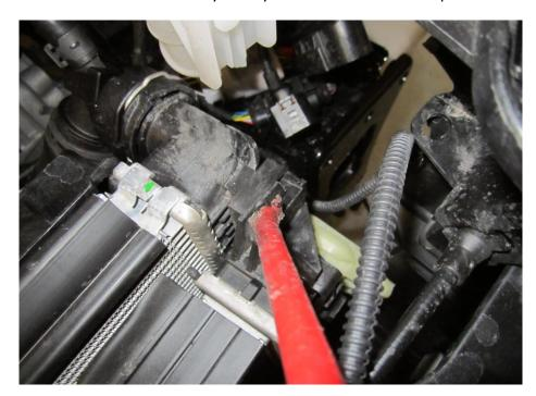
30. With the intercooler removed you need to trim the plastic cowl where the new intercooler sits. This can be done with a dremel, sharp knife or similar.
