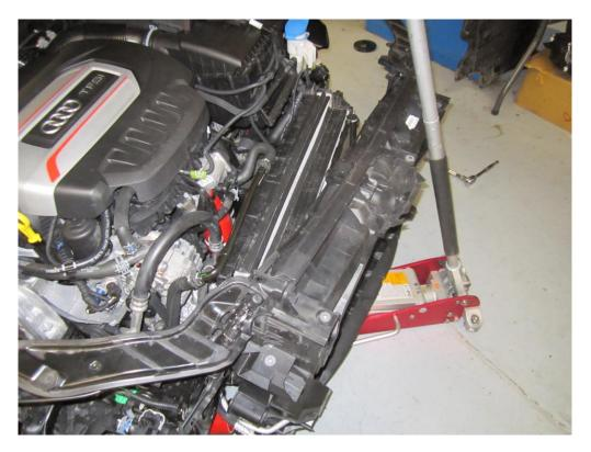
29. Using a flat bladed screwdriver, push down on the tabs holding the radiator to the intercooler. Push the radiator away from you while the tabs are depressed.
