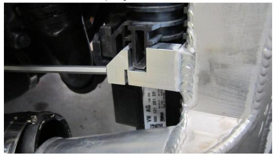
34. Pull the top of the radiator towards you and locate the top tabs of the radiator into position .
