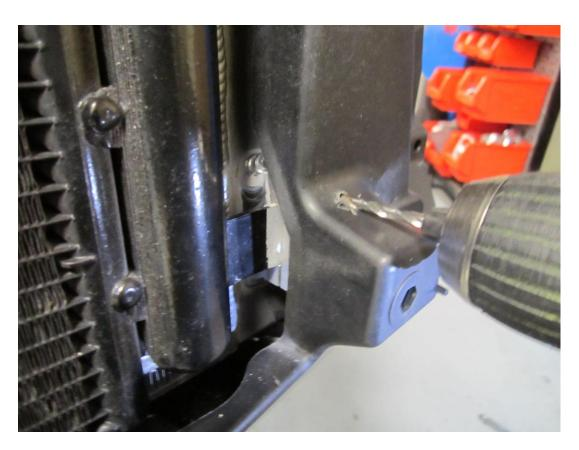
38. The fasteners on the left hand side of the cowling (when viewed from the front of the vehicle) need no holes as these can be tightened using exsiting access and a ball ended 3mm allen key.
