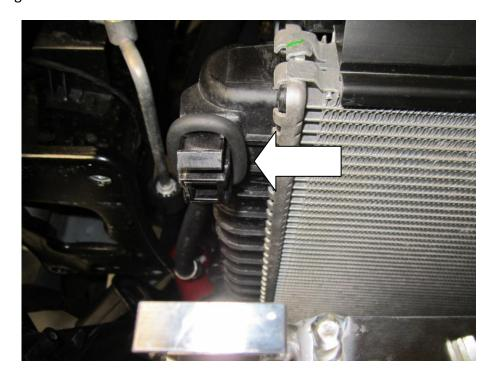
32. Loosen but dont remove the lower brackets on your new intercooler using a 6mm allen key.
