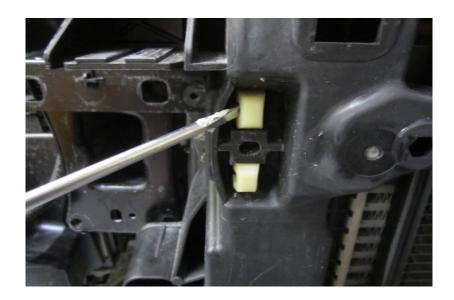
25. Using your T27 torx drive, remove the last two fasteners holding the radiator cowling into place. These are located next to where the lights where located.
