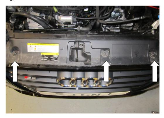
4. Using your T45 torx drive undo the three fasteners at the rear of the under tray .
