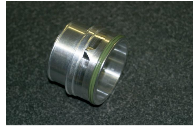
16. Carefully remove seal from original hose and install on NEUSPEED billet hose coupling.
