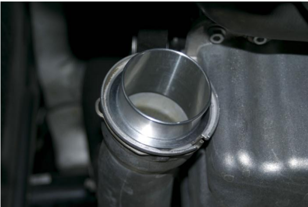
17. Install NEUSPEED billet hose coupling into OE aluminum pipe. Make sure clip locks into place.
