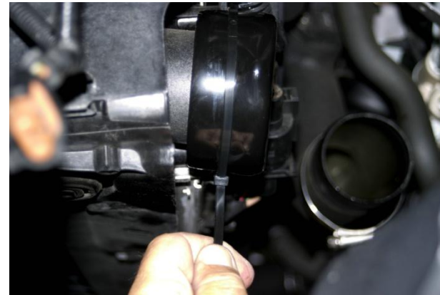
20. Using supplied cable tie, install black cap on outlet side of original intercooler.
