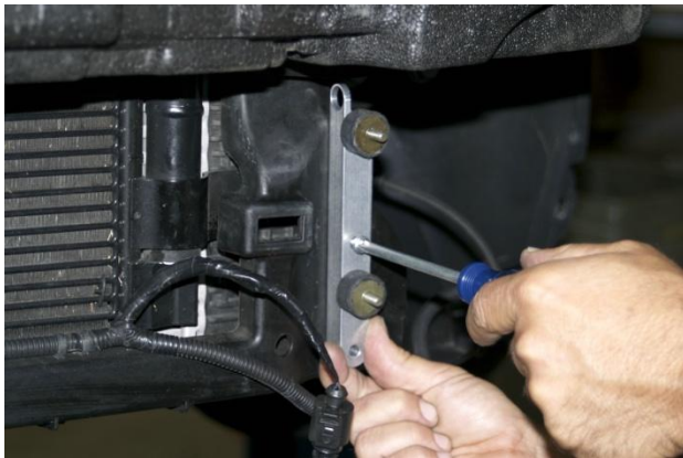
11. Using supplied #10 sheet metal screws and lock washers, attach intercooler mounts to existing holes in radiator core. Mount with sensor hole provision on top, mounts to driver's side of vehicle.
