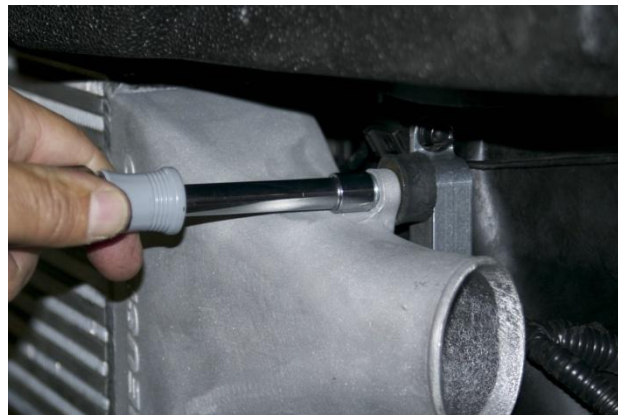
12. Install outside temperature sensor onto driver's side mount and remove wire harness and retaining clips from sides of radiator core. Using supplied cable ties, tie the harness to radiator core as pictured.
