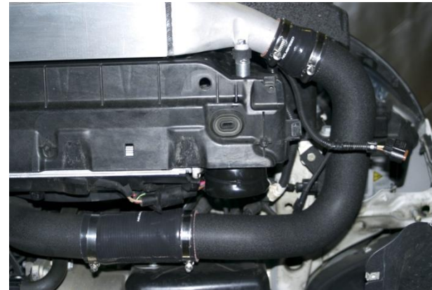
21. Assemble and install intercooler outlet pipe and hoses as pictured with supplied clamps using silicone hose reducer, custom aluminum pipe and 6" silicone hose. NOTE: Adjust pipe as necessary for fog light clearance. Tighten all hose clamps with 7mm nut driver.
