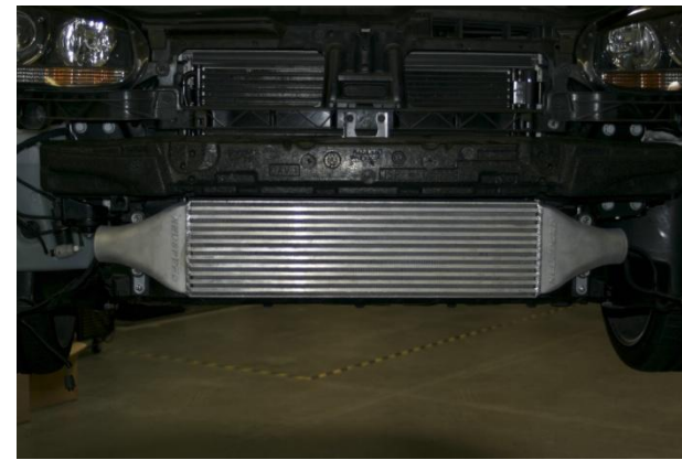
13. Mount intercooler core to vehicle using the supplied (4) 10mm hex flange nuts.
