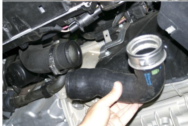
19. Remove the driver's side intercooler hose. Using a screwdriver, pry out locking spring clip to release hose at the intercooler and undo clamp at pressure pipe.
