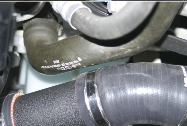
18. Assemble and install intercooler inlet pipe and hose section as pictured with supplied clamps. NOTE: NEUSPEED print on 45° hose goes toward billet coupling. Adjust hose connections as necessary for clearance. Tighten all hose clamps with 7mm nut driver.
