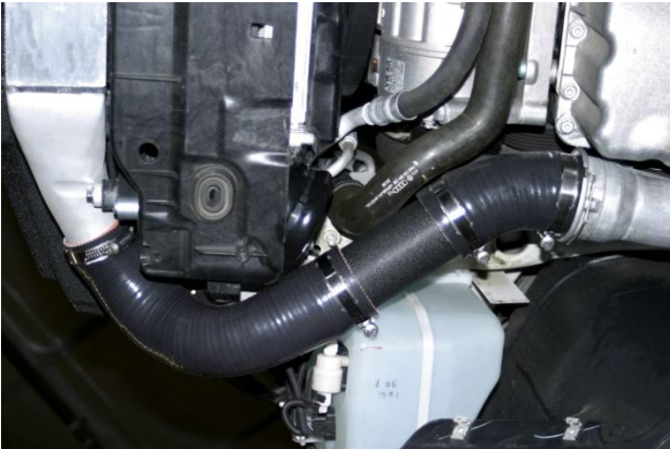
17. Install NEUSPEED billet hose coupling into OE aluminum pipe. Make sure clip locks into place.
