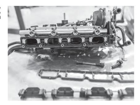
32) Install the supplied plug in the end of the runner flap assemble and reinstall the original clip to hold it in place.
