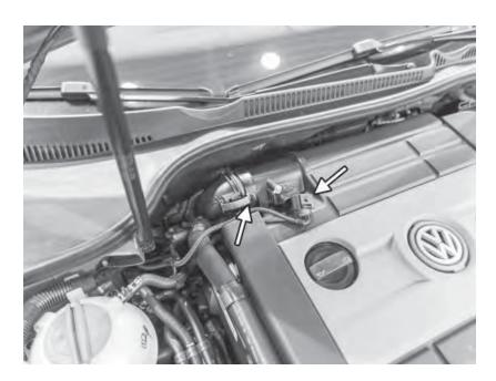
53) Reconnect the MAF sensor electrical connector and install the plastic compressor inlet hose to the airbox.
