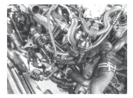
26) Carefully remove the intake manifold assembly, making sure there are no other lines or wires that are connected. The fuel pump and fuel lines will come off with the manifold. Make sure that the o-rings from the stock fuel injectors are not in the intake manifold.
