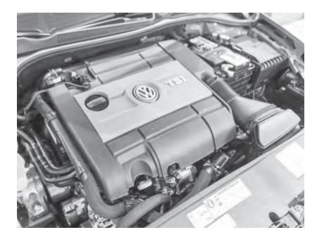
52) Reinstall the two T25 screws that connect the intake ducting to the radiator support. Reinstall the hose clamp next to the round accordion tube.
