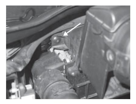
2) Open the hood and remove the two T25 screws that connect the intake ducting to the radiator support. Then remove the hose clamp next to the round accordion tube, and remove the intake from the car.
