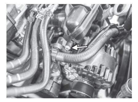
18) Remove the 10mm bolt from the passenger side of the intake manifold coolant pipe.
