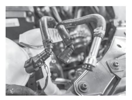
17) The two plastic fittings are disconnected by pushing in on the side of the fitting and lifting the connector off from its mounting location. The metal fitting is removed by lifting the plastic up into the metal housing, and then lifting the line off. The metal fitting is a fuel line, so be sure to use a rag to keep from splashing fuel everywhere.
