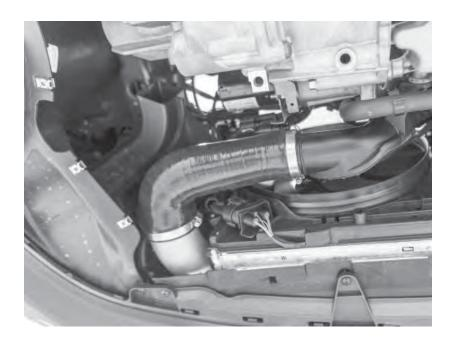
49) Reconnect the lower intercooler hose to the intake charge pipe and tighten the hose clamp. Also tighten both hose clamps to the rubber boot off of the throttle body. Reinstall the belly pan on the vehicle.
