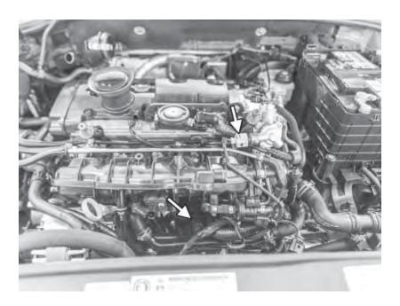
41) Connect the following electrical connectors on the intake manifold: plug under the intake manifold by the alternator, connector to the variable intake runner control, the wiring harness clip on the fuel line, EVAP purge valve, fuel pressure sensor, fuel pressure regulator, and fuel injector wiring harness.
