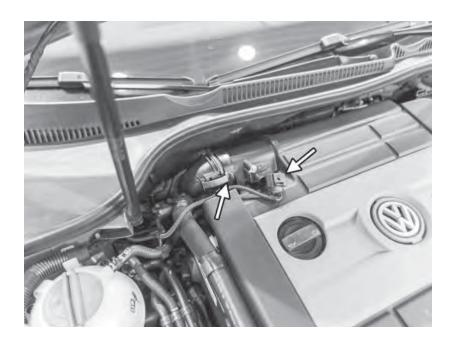
4) Remove the two clips for the diverter valve hose from the right side of the airbox/engine cover. Remove the factory airbox assembly from the engine by lifting on the cover in the following order: Left Front, Left Rear, Right Rear, Right Front. The airbox will come out easily if done in this sequence. There are four rubber grommets that connect the airbox to the engine. Make sure they are still attached to the airbox.
