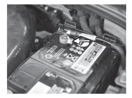
54) Reconnect the negative battery terminal. Let the car sit for at least three minutes with the igniton on and the engine off. This is also a good time to connect to the car with a diagnostic tool to clear any error codes on the car.
