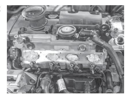
28) On the left side of the intake manifold, disconnect the metal clip from the runner flap lever. Also gently pop off both socket ends from the connecting rod linking the runner flap motor to the runner flaps.
