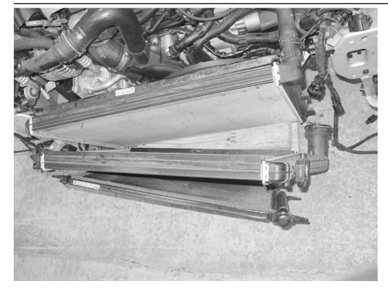
27) Carefully maneuver the stock intercooler out of the car from between the condenser and the radiator.
