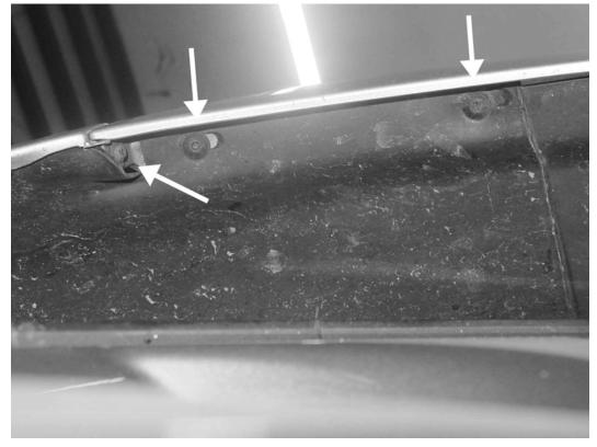
5) Remove the T25 Torx Screws that run along the inside of the front of the wheel wells. These connect the fender liner to the bumper. Also remove the two screws that connect the bumper to the fender.
