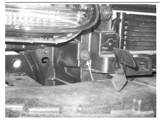
35) From the front of the core support, attach the two T30 screws that connect the intercooler side grommets to the radiator core support.
