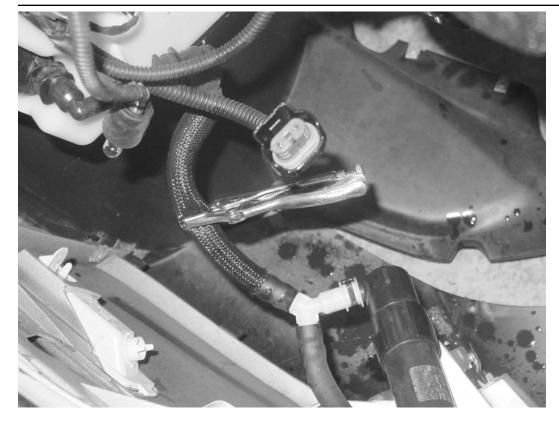
9) With a partner, slide the bumper cover forward several inches. Clamp the headlight washer line before the "T" with a suitable tool to prevent washer fluid loss. Remove the washer lines from the clips at each washer, and separate the line from the clips in the bumper.
