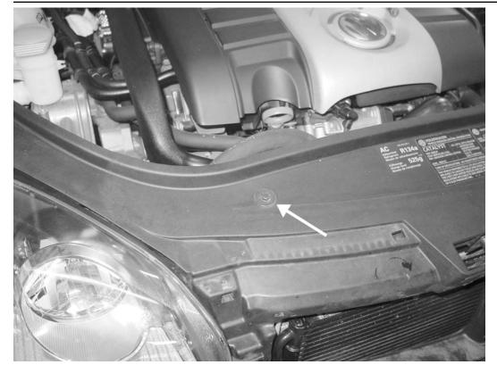
13) Remove the 8mm bolt that connects the noise booster to the upper radiator support.
