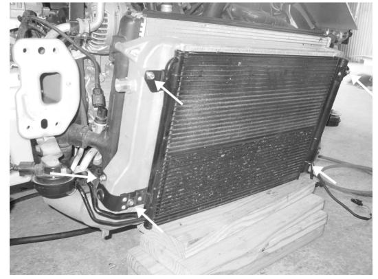
29) Connect the condenser to the APR intercooler using the five 10mm bolts. These five bolts connect the condenser to the APR intercooler in the same locations as the stock intercooler. Be sure to install the side condenser hose bolt first before trying to install the four bolts on the front of the condenser.
