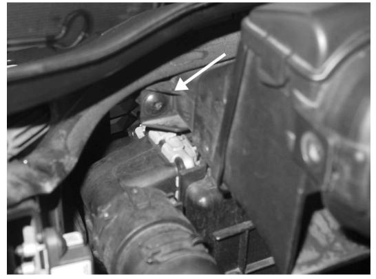
3) Remove the two T25 screws that connect the intake ducting to the radiator support. Then remove the hose clamp next to the round accordion tube, and remove the intake from the car.
