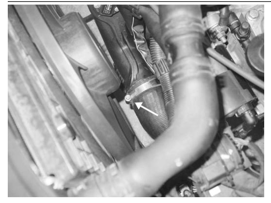
21) Loosen the hose clamp on the passenger side intercooler hose from above the car.
