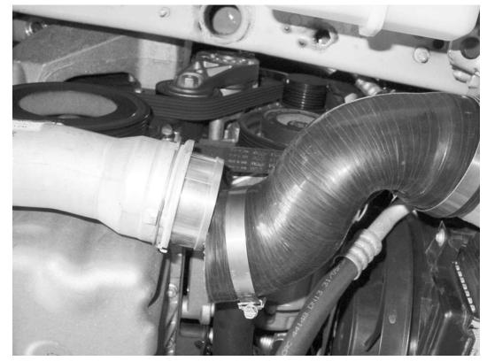
45) Making sure the locking clip is pulled away from the stock coupling on the car, install the APR coupling adaptor. Then install the APR passenger side intercooler hose using the two supplied hose clamps. Connect the two ends of the hose, make sure the hose is oriented without any kinks, and tighten both hose clamps in place.
