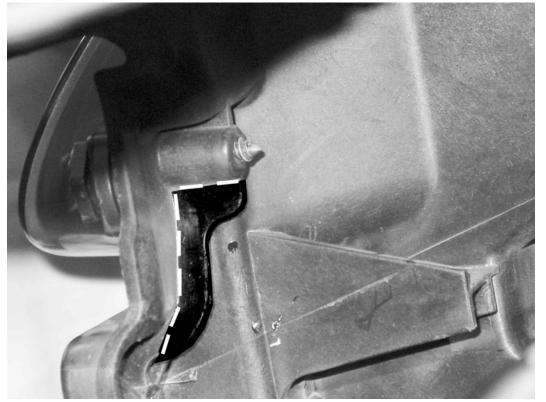
31) On the radiator core support just above where the side intercooler grommets mount, you must trim off the excess plastic outlined in the picture. Otherwise, the upper condenser to intercooler bolts will hit the core support. The plastic is easily cut with snips or side cutters.
