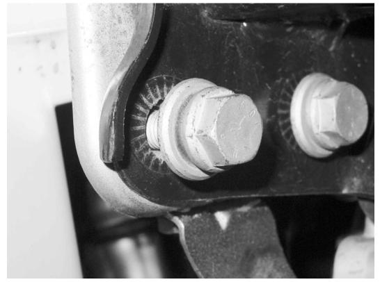
41) With help from a partner to support the radiator core support, tighten the 16mm bolts while trying to align the heads of the bolts with the marks from where they were previously installed. Tighten the upper T25 fender bolts at this time too.
