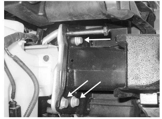
15) Remove the remaining six 16mm bolts from the car and carefully pull the radiator core support forward an inch or two. Be careful not to stretch the two air conditioning lines located on the passenger side of the A/C condenser.
