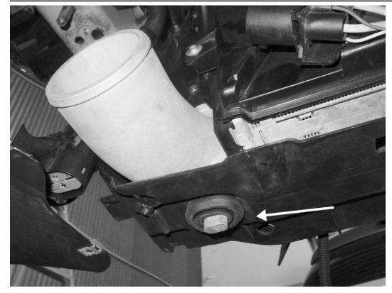
33) From underneath the car, lift up on the intercooler/condenser/ fan assembly and set the bottom "feet" of the APR intercooler into the rubber grommets on the core support.
