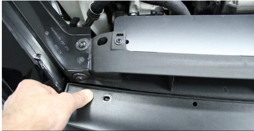
36. Now push the top of the grill back under the slam panel no both sides.
