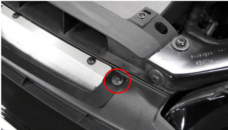
38. Secure this side too – the screw should go through the scoop surround.
