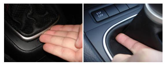
Position the shift lever so that the two alignment holes allow you to position the included nail into the holes as show below thus locking the lever in place.
