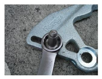
For the side-to-side linkage, the procedure is the same. You will need to select the cable shaft that matches your OEM linkage and attach it using the supplied 13mm lock nut. Position the shaft at your desired adjustment location and tighten it securely in that position.
