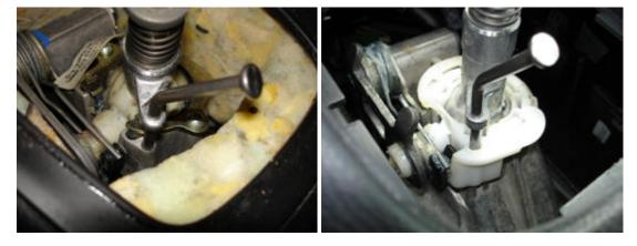
Returning to the engine bay and the shift linkage components, for MK4 VW 6-speed applications, you will need to press down slightly on the linkage from its neutral position as well as locate a small black pin on the side of the transmission just below the linkage.
