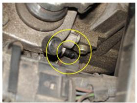
(For MK5 applications, this locking pin is not incorporated on the transmission casing so the linkage will need to be kept in its normal neutral position.)
