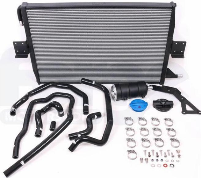
This kit has been developed to fit the Audi S4 3.0TFSI fitted with **Twin** chargecooler radiators. As well as the OEM chargecooler radiator there is also a side mounted chargecooler radiator.
