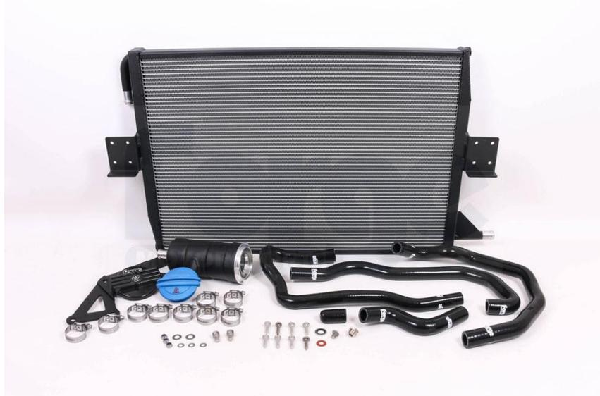
This kit has been developed to fit the Audi S4 3.0TFSI fitted with a **Single** OEM chargecooler radiator. The OEM chargecooler is located in front of the main radiator. This comprehensive kit allows the engine and chargecooler coolant to be separated as well as the improved cooling of the larger chargecooler radiator, giving better control over chargecooler coolant temperatures and recovery times. This kit is supplied with a CNC machined billet Forge expansion cap cover.
