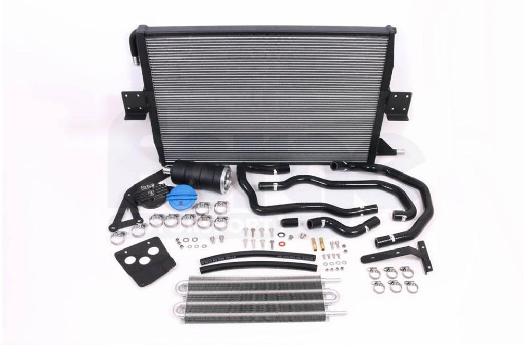
This kit has been developed to fit the Audi S4 3.0TFSI fitted with a **Single** chargecooler radiator **and optional ADS** (Audi Dynamic Steering) oil cooler. These vehicles are fitted with a large oil cooler located in front of the main radiator. Using the parts supplied in this kit the OEM oil cooler is replaced and relocated.
