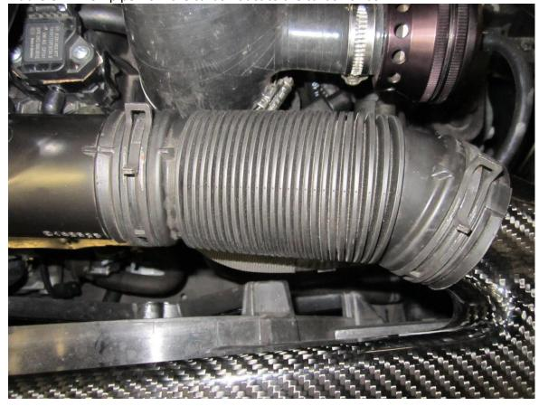
**16.** Tighten the hose clamps on the turbo inlet pipe, being cautious not to over tighten the hose clamp on the carbon fibre lid as this could crack and fracture if over tightened.
