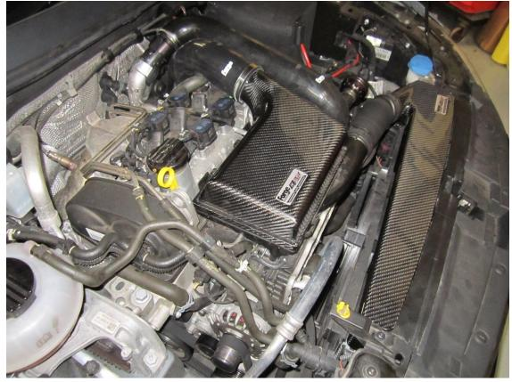
14. Fit the carbon fibre enlarged front duct into position using the 2x M6 fasteners provided.
