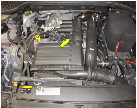
**5.** Remove the front air scoop and remove the airbox by pulling it sharply in an upwards motion.
