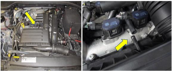
4. Remove the hose clamp that holds the airbox to the turbo inlet hose.
