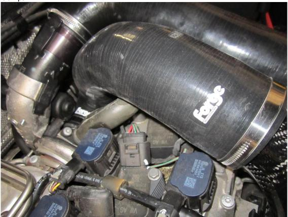
**13.** Use silicone spray in the end of the turbo inlet pipe to help when fitting the airbox into situ not forgetting to connect the engine breather to the airbox.
