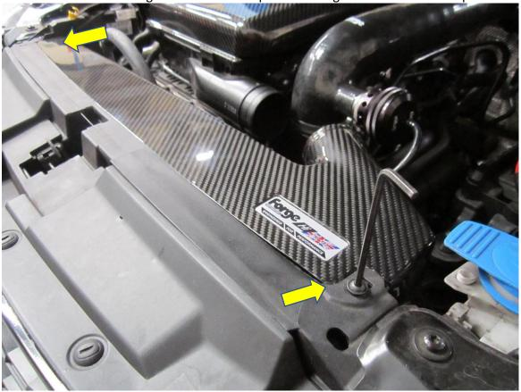
**15.** Fit the OEM flexi pipe from the carbon duct to the carbon airbox.
