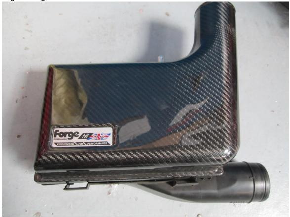
**12.** Fit the large bore high flow turbo intake into position but do not tighten the hose clamps.
