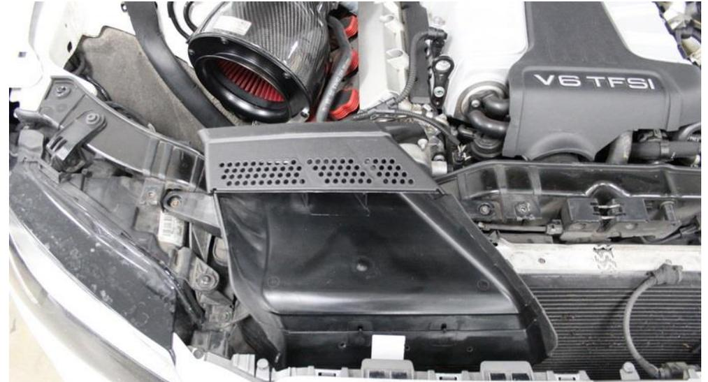
34. For pre-face lift S5's: Place the stock duct in place and secure with the 2 screws previously removed.
