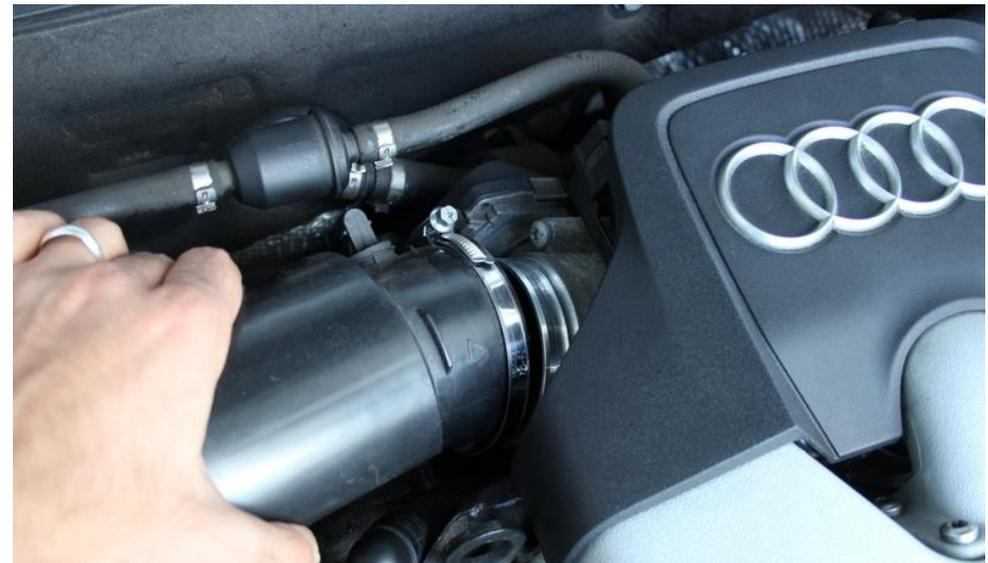
8. Loosen hose clamp around the throttle body and pull the tube away.
