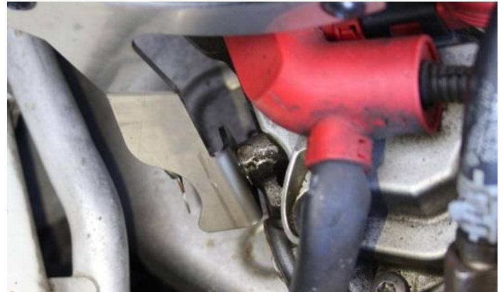
20. Line up the housing so that the bracket meets the mount as shown. Hold it in this position and tighten the hose clamp around the tube as shown in next step.
