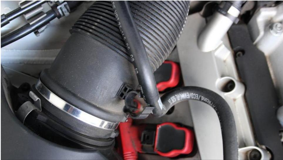
5. Remove the hose from the intake tube.
