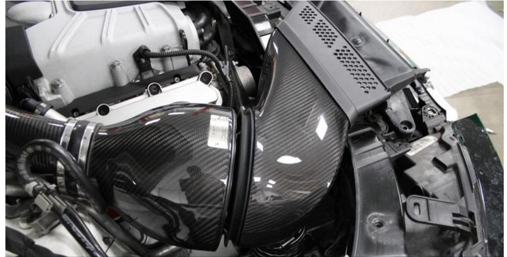
46. Keep pushing the flexible tube down until you can line up the carbon duct with the carbon housing. The metal cowl at the mouth of the filter should go inside the carbon duct. Be careful not to pull the rubber edging on the duct out of position. If this does happen – pull the duct back out and re-align the rubber edging.
