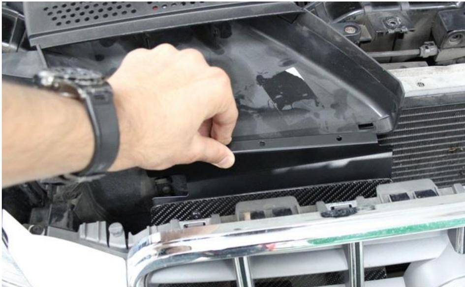
31. Place the scoop assembly into position so that the 3 slots on the metal scoop extension sit over the stock duct edge.
