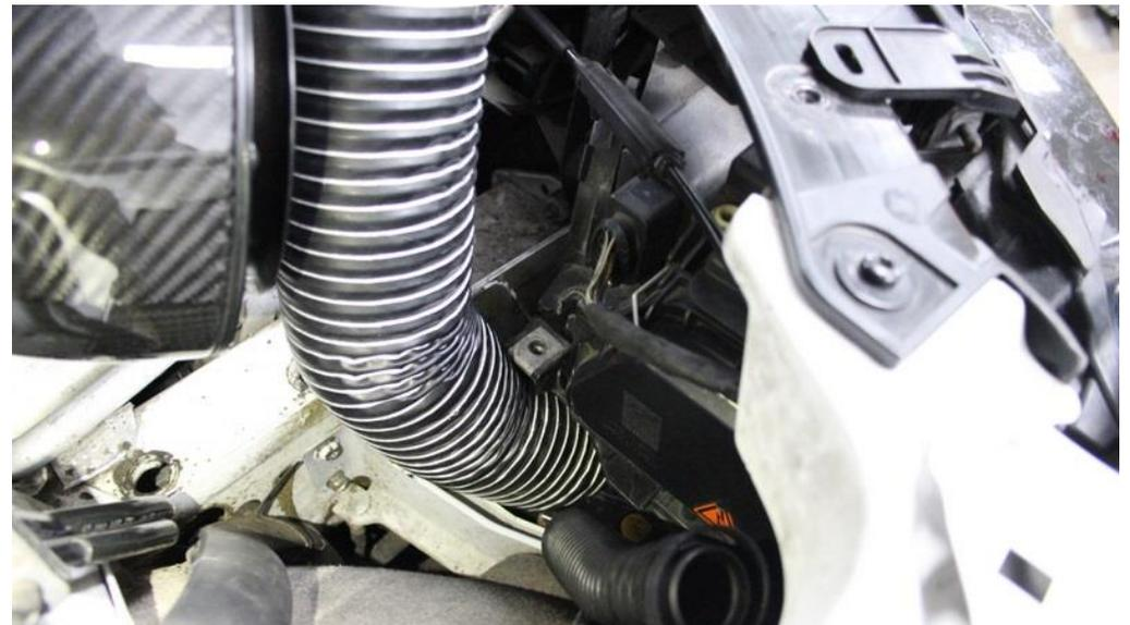
44. Feed the flexible tube underneath the headlamp - see next step.
