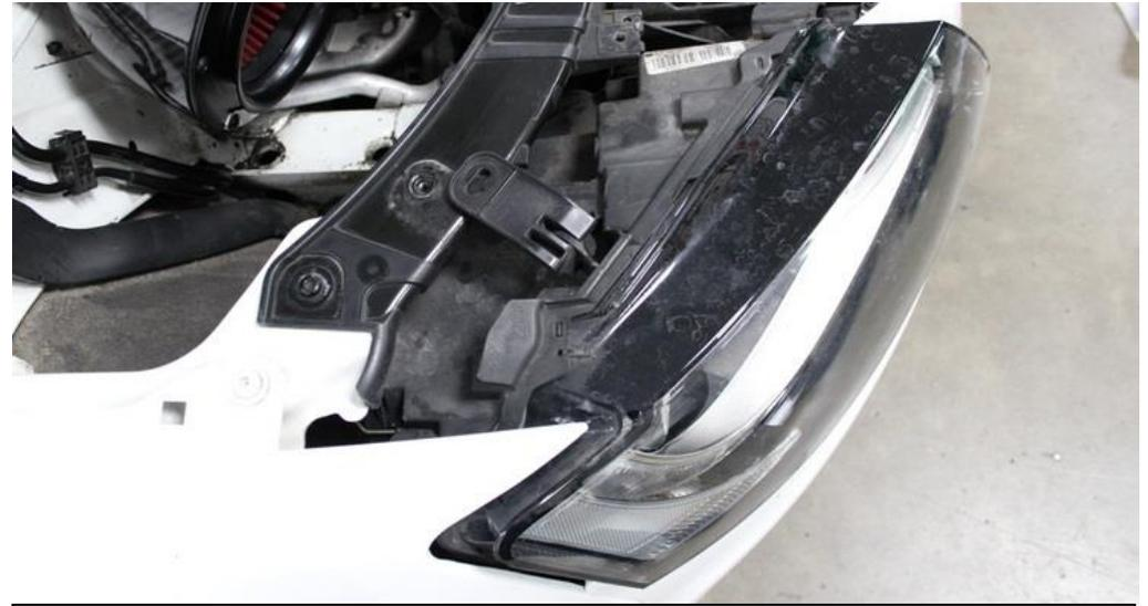
42. Now carefully move the headlight out by a couple of inches. Just enough to allow the flexible duct to be positioned.
