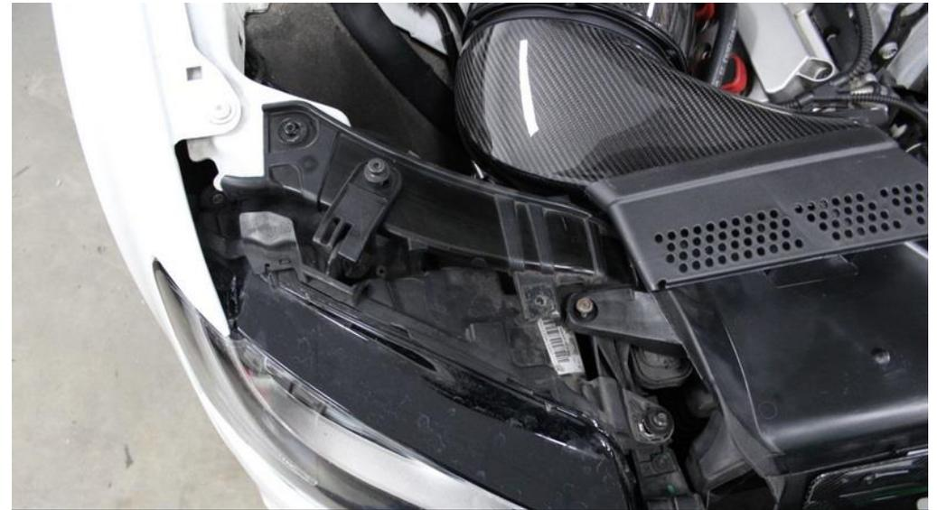
50. Now carefully push the headlight back into position and secure the 3 previously removed screws.
