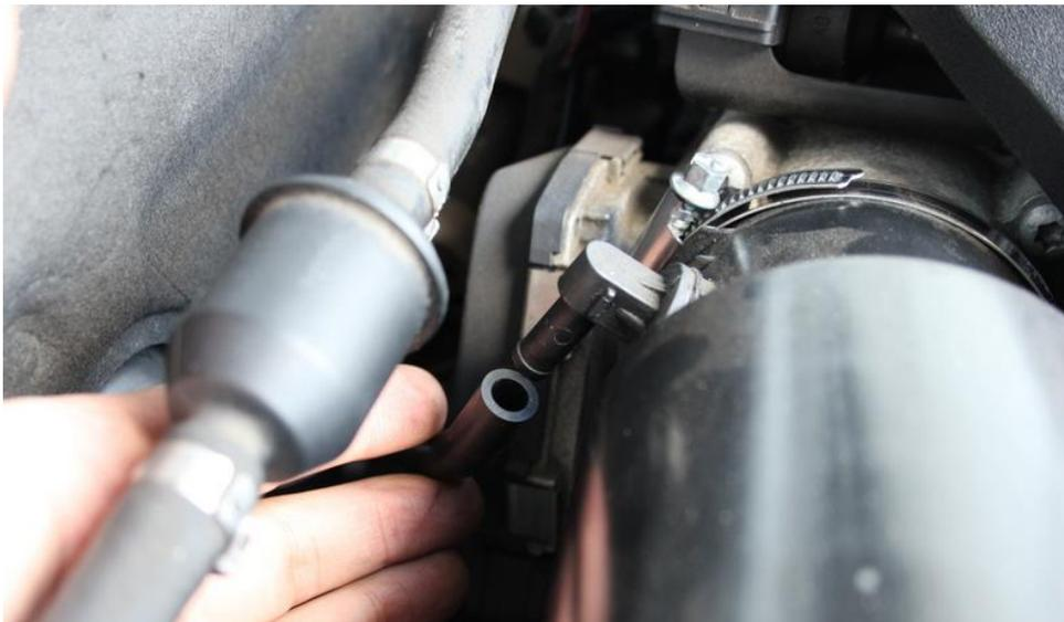
7. Pull the vacuum out from the back of the intake tube next to the throttle body.
