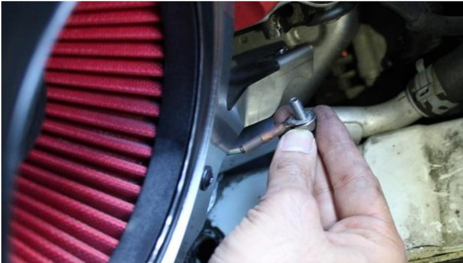
23. Push the earth cable over the bolt as shown and then push the bolt through the hole in the bracket and into the threaded mount on the engine. Screw the bolt in but don't fully tighten yet – you need to adjust the position of the housing.
