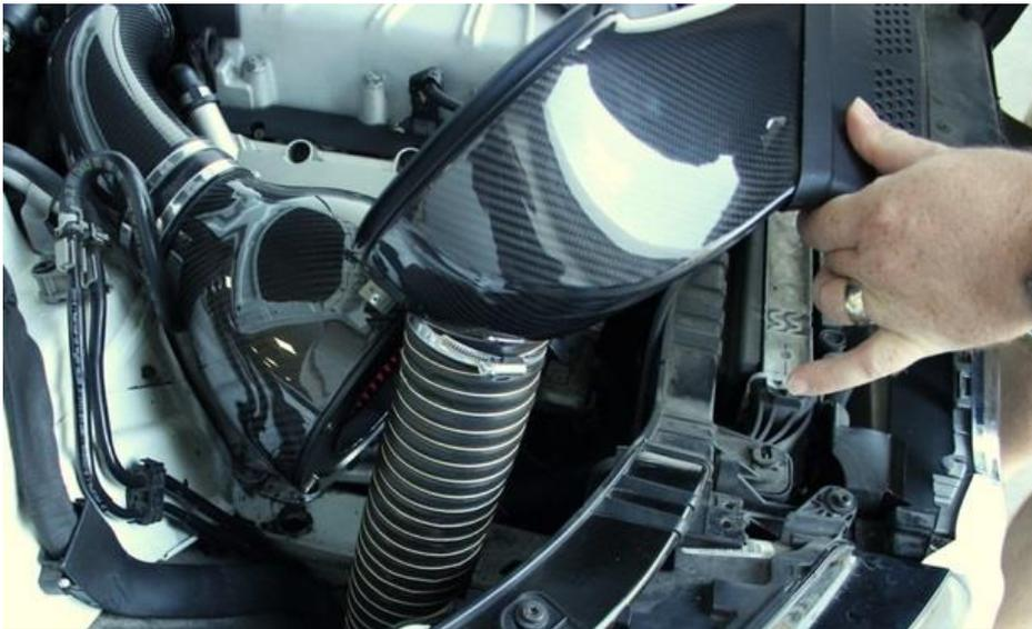
43. Take the duct assembly and lower the flexible tube behind the headlight.
