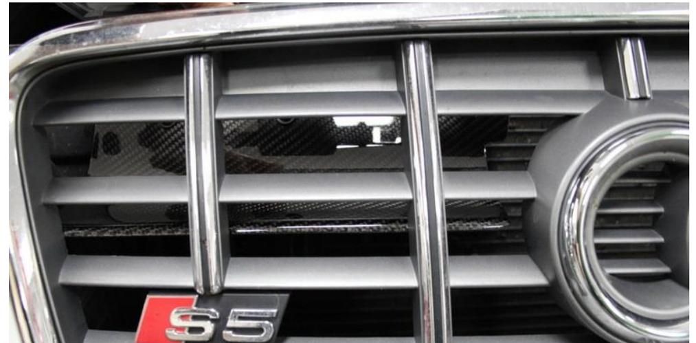
36. Position the scoop so it sits against the grill – avoiding any obstructions. Once in position, mark and drill 3 holes in the stock duct through the 3 holes on the scoop using a 5mm drill bit. Do not secure the scoop to the duct yet.
