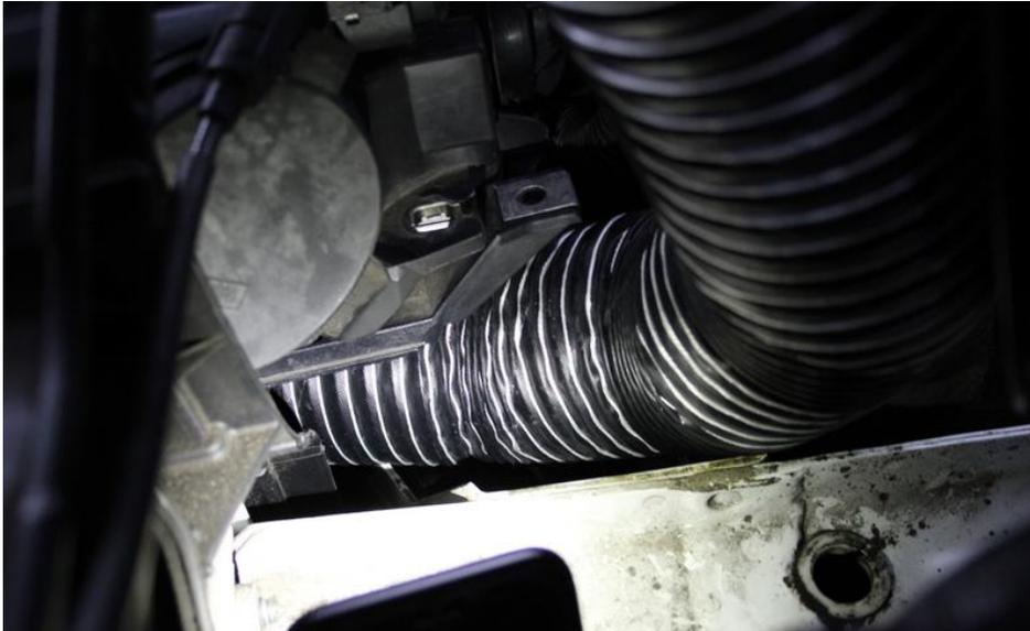
45. Push the tube under the headlight and keep feeding it as you lower the duct. The tube should be near the front bumper area.
