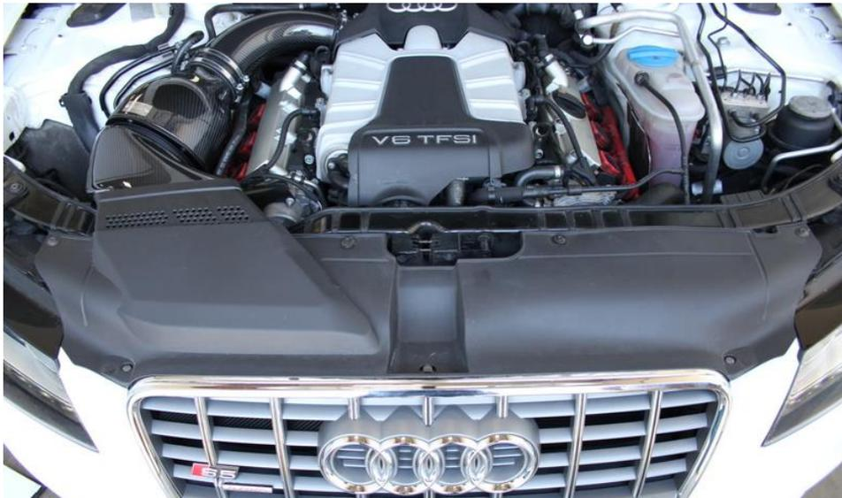
55. Install the slam panel cover and secure with the screws/plugs previously removed.
