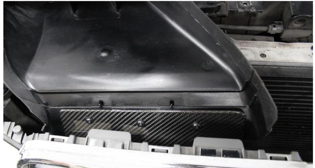
48. For the pre-face lift version, lower the scoop into place and secure with 3 black screws and lock nuts.
