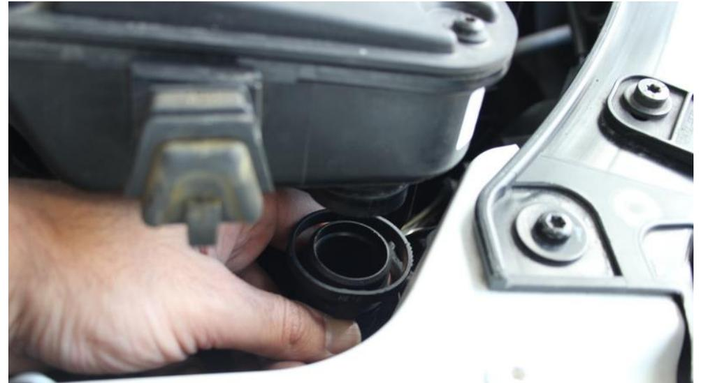
10. Disconnect breather tube from the airbox by pinching in two side of the flange around the tube to release the clips. The airbox can now be pulled upwards and removed from the engine bay.
