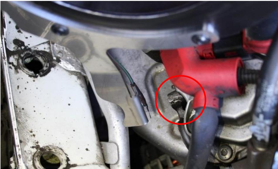
19. Here is another angle with the mounting point circled in red. Rotate the housing so that the bracket meets the mount. See next step.
