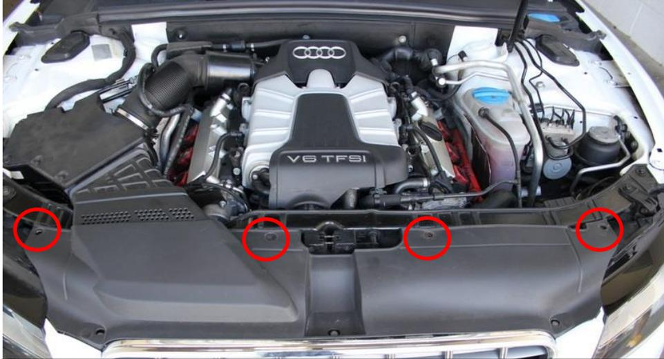
1. We will start by removing the front slam panel cover. Remove the clips/screws holding the cover in place and remove the cover from the engine bay.
