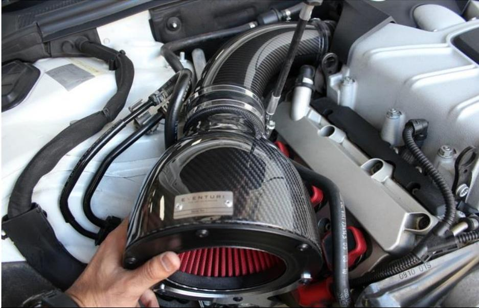
21. Holding the housing in place, secure the hose clamp around the tube where it meets the housing. Do not over tighten.
