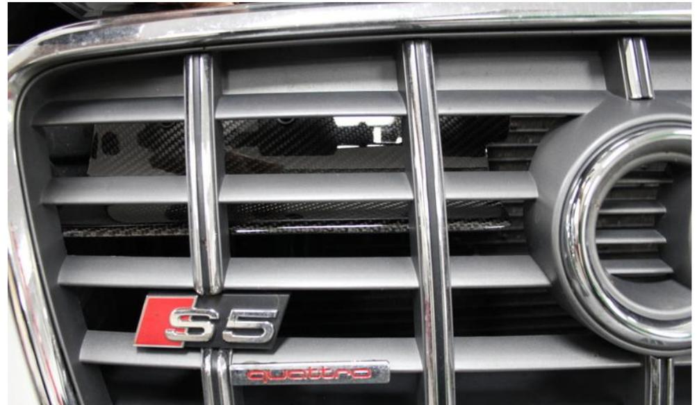
32. Position the scoop so it sits against the grill – avoiding any obstructions. Once in position, mark and drill 3 holes in the stock duct as shown in next step.
