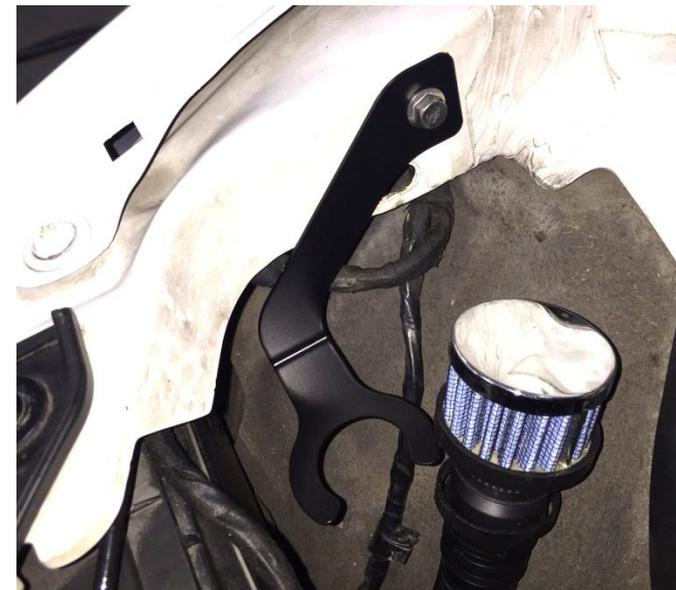
52. Push the breather assembly onto the secondary air pump tube – it will click into place. Also secure the breather filter bracket to the chassis using the previously removed screw in step 11.
