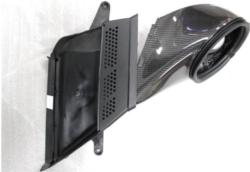
37. Take the stock duct and the carbon duct – insert the right side corner into the plastic duct as shown and then push the rest of the carbon duct into the stock plastic one. It should click securely into place.
