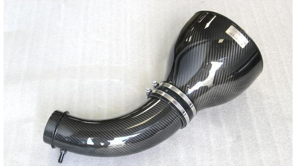
14. Now push the carbon intake tube into the silicon hose as shown. Lightly secure the hose clamp around the tube – the tube should still be able to rotate. We will fully secure it later.
