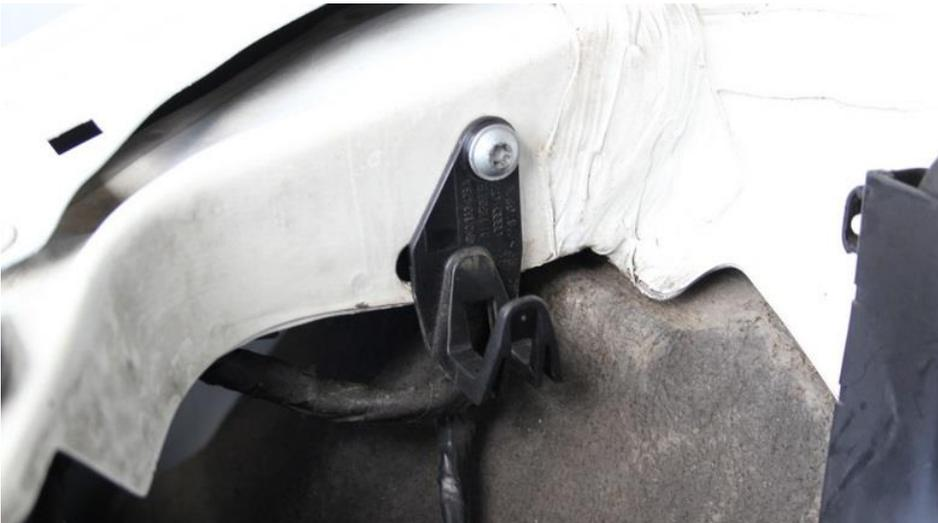
11. Remove this bracket which held an airbox mount. Retain the screw for use later on.
