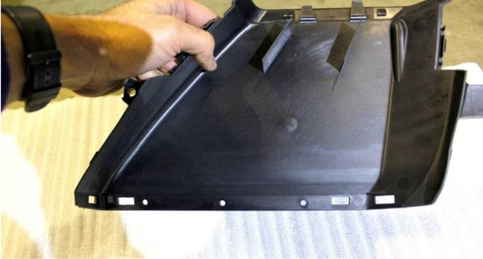
33. Use a 5mm drill bit to make 3 holes in the stock duct using the slots in the metal scoop extension as a guide. Do not secure the scoop to the duct yet.
