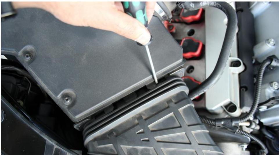
3. Using a screwdriver – carefully release the rubber duct from the airbox by pushing down the tabs.
