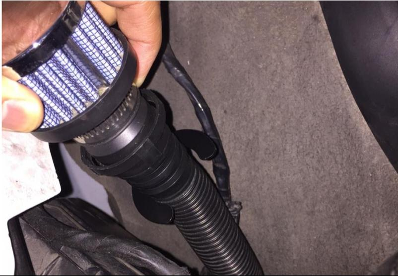
53. Pull the breather filter upwards so that so are able to push the flexible air pump tube into the bracket.
