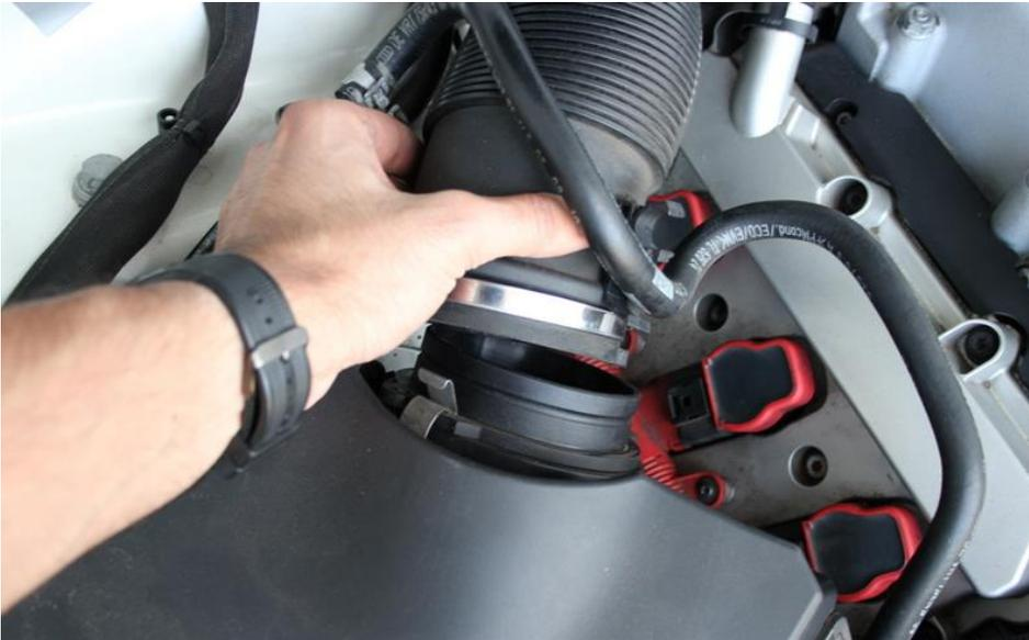
9. Remove the inlet tube from the airbox side too and completely remove from the engine bay.
