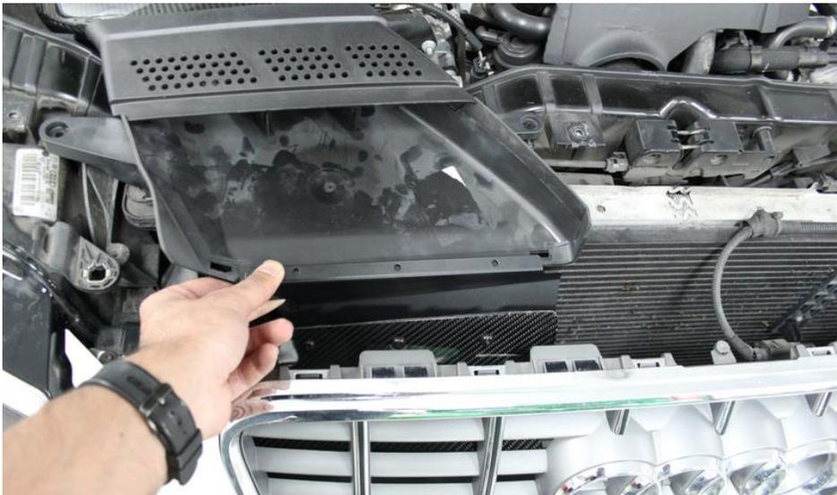
47. Now position the scoop assembly over the holes previously drilled and secure with 3 black screws and lock nuts. Photo shows facelift version.
