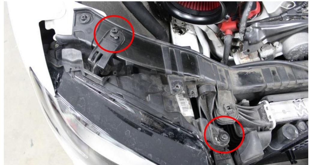
40. The flexible tube will sit underneath the headlamp – for ease of installation, we will move the headlamp forward. Remove the 3 screws holding it in place. 2 Shown here.
