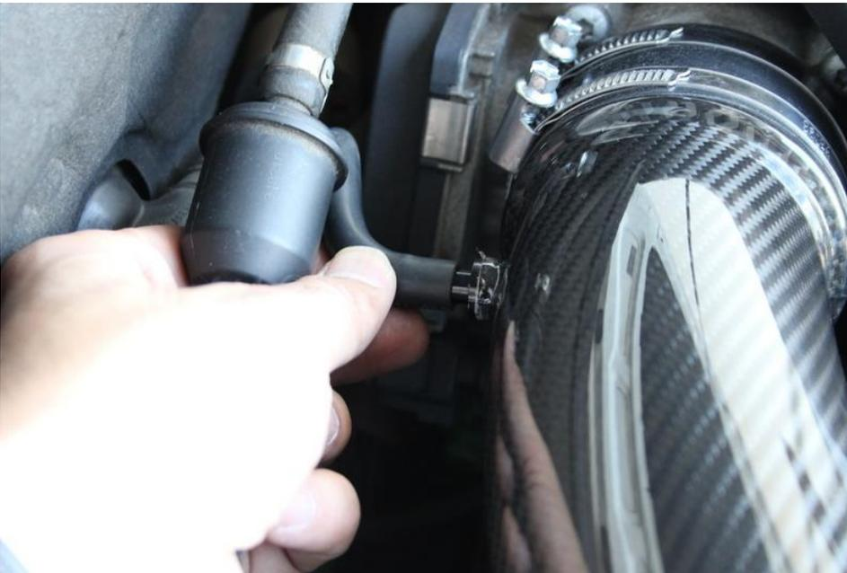
27. Push the boost/vacuum line onto the tube.
