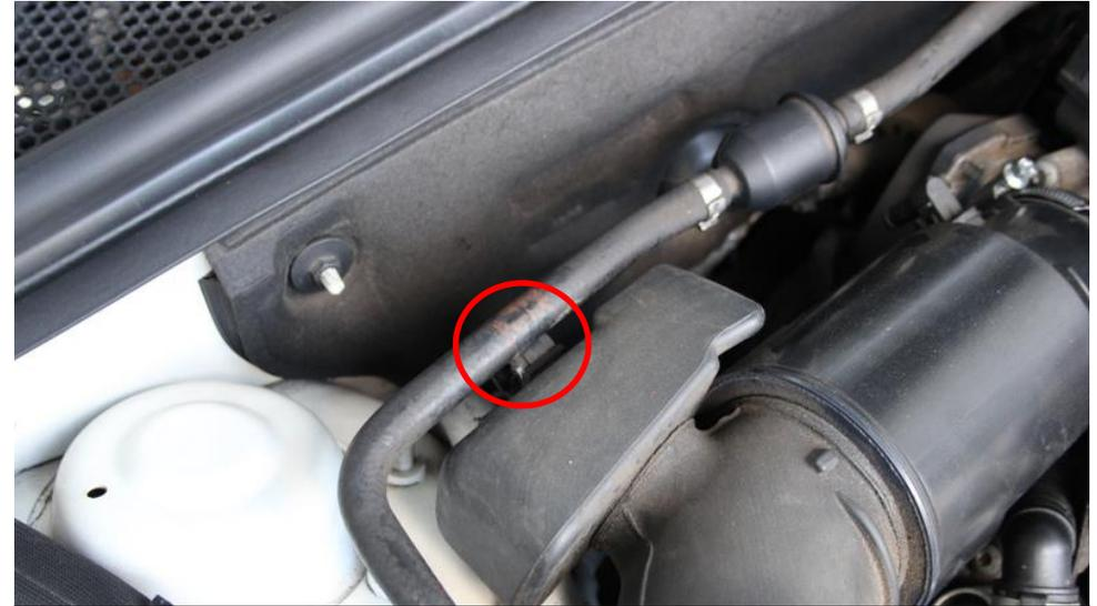
6. Remove the hose at the rear from the silencer box on the tube.
