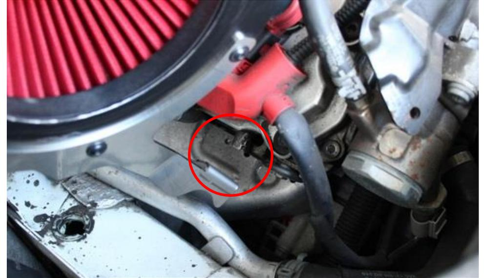
18. The flange on the bracket needs to line up with the mounting point where the earth cable was attached.
