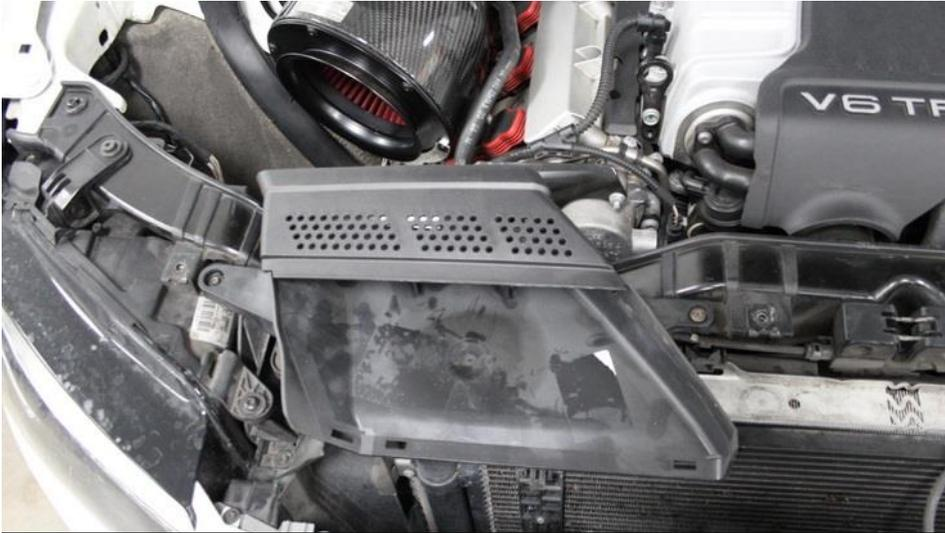
29. For facelift S5's: Place the stock duct in place and secure with the 2 screws previously removed.
