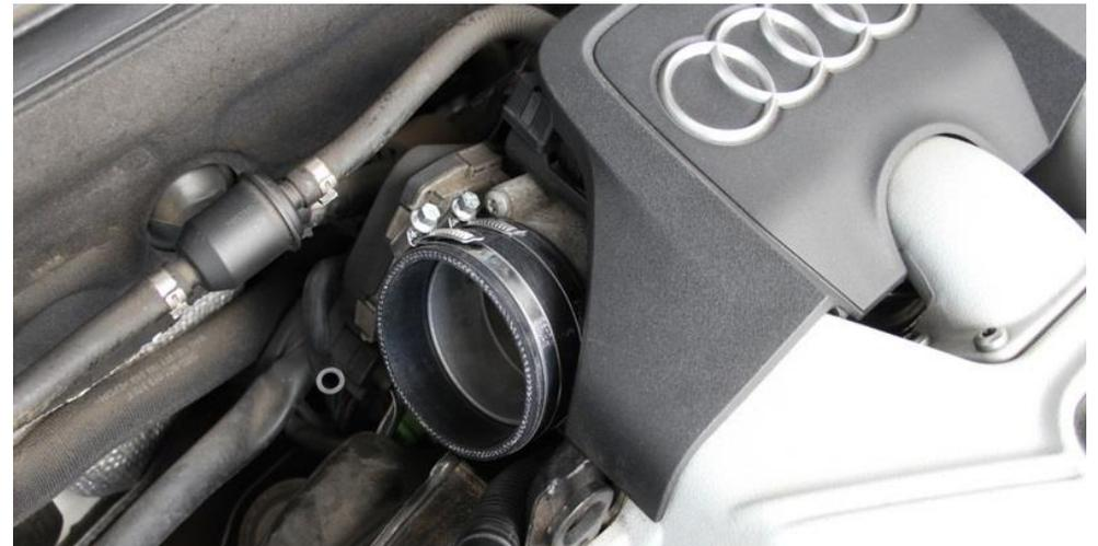
12. Push the smaller silicon coupler over the throttle body. Ensure it is fully on and uniform all the way around. Use 2 x 70-90mm hose clamps as shown and secure the hose clamp around the throttle body.
