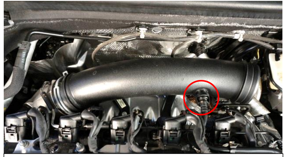
6. Remove the spring clamp holding the turbo tube to the rubber joiner and also the breather connector circled in red.
