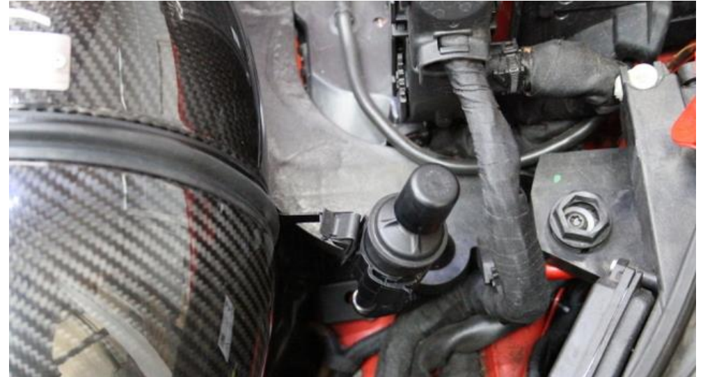
43. Push the sensor pot onto the small bracket extending from the housing
