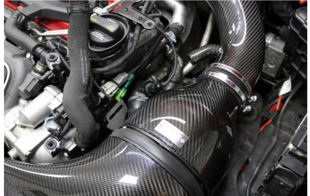
35. Rotate the housing so that the brackets line up – see next step. Ensure the rubber cushion on the duct is sitting squarely on the housing.
