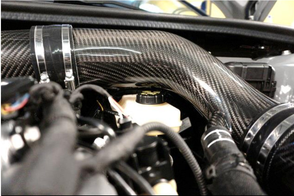
34. Position the tube so that it clears the brake fluid reservoir (LHD models only). It should have about 10mm clearance.
