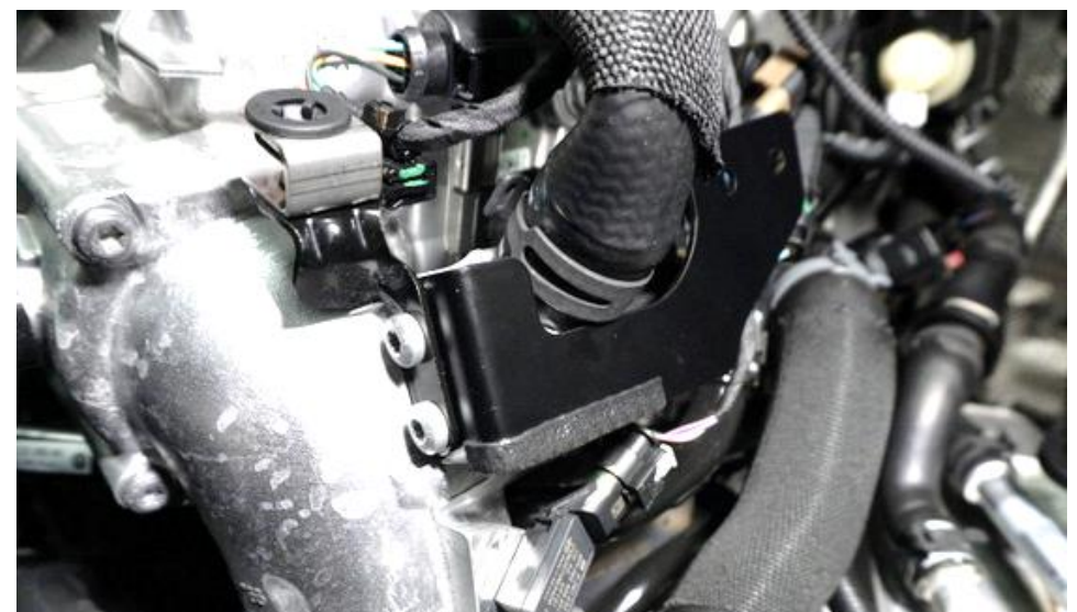
20. Install the new bracket for the intake as shown. Put the original bracket from the previous step on TOP of the new bracket and secure with the same 2 Torx screws.
