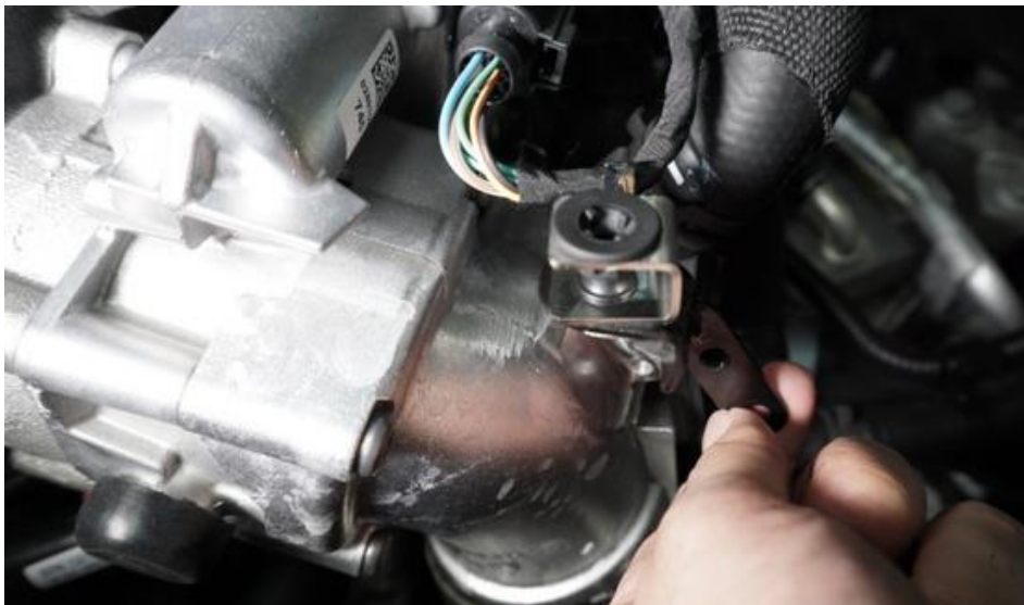
19. Now push the rubber mount back into the new bracket.
