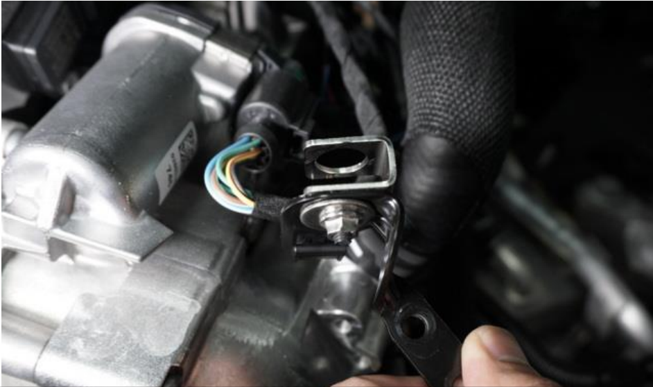
17. Install the Spacer bracket using the supplied M5 screw, M5 nut and washer. The nut and washer should be at the bottom of the bracket.
