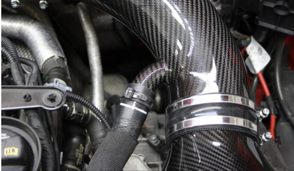
42. Push the breather onto the carbon tube and secure with the original spring clamp.
