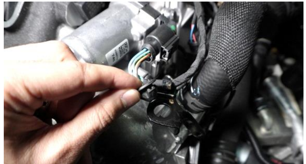
16. (STEPS 16 to 19 are not necessary for the RS3 – only for the TTRS) Remove the rubber mount on the bracket from the previous step. We will install a spacer bracket to raise the engine cover for more clearance.
