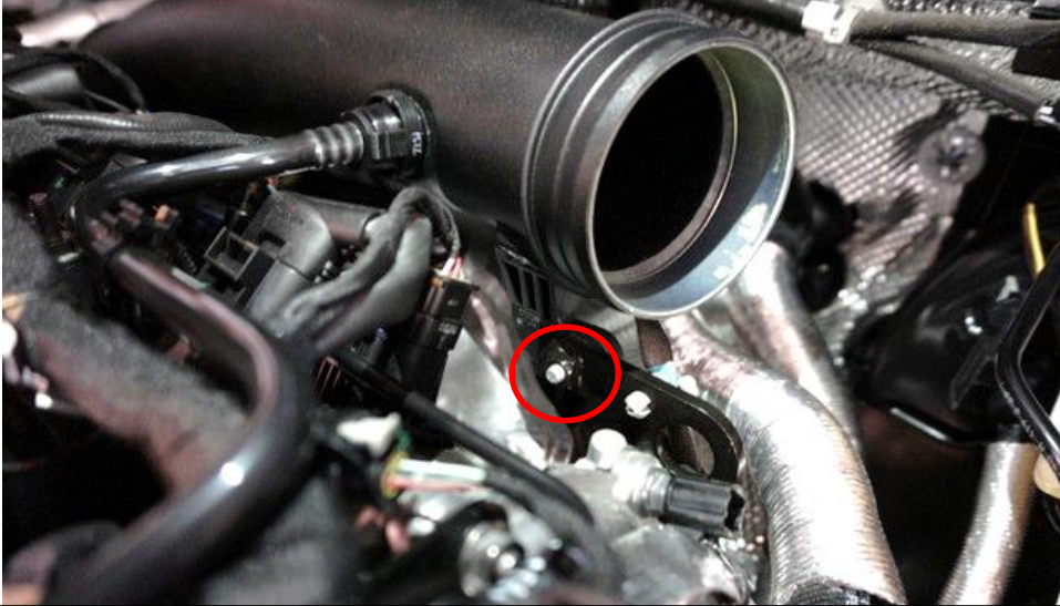
5. Remove the screw securing the Turbo Tube.
