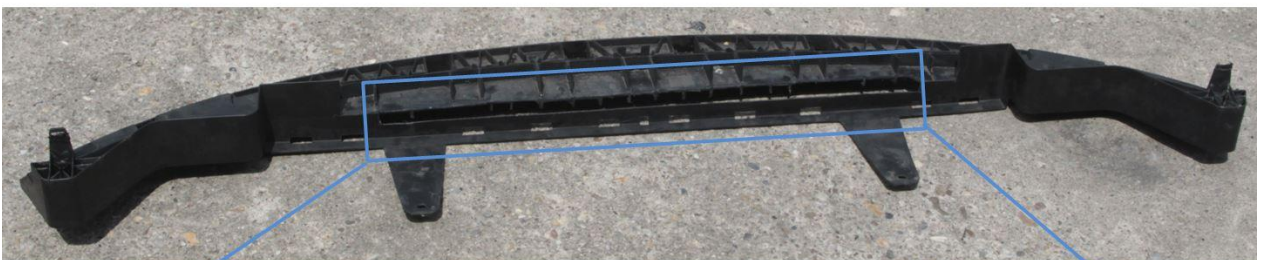
Cutting the plastic inside the bumper.
