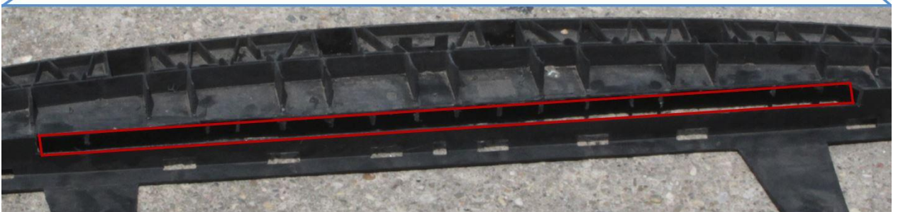
Cutting the plastic inside the bumper.
