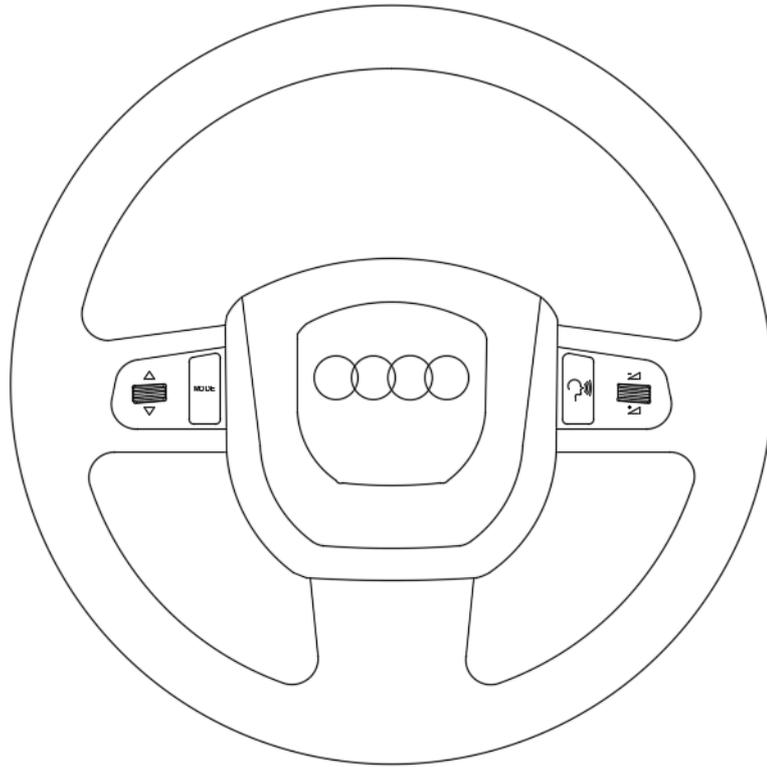
Para move up and down in the Polar FIS screen you should turn the wheel in the left side
