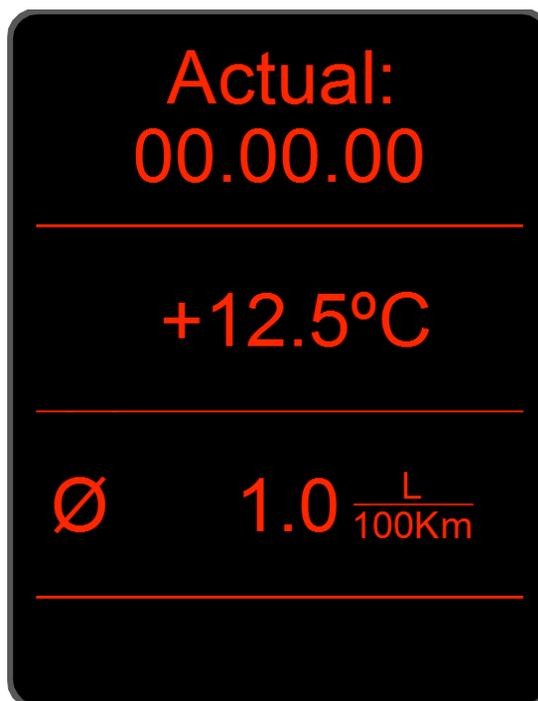
If after a measure you want to do another one, it is not necessary to exit from stopwatch screen, simply press the OK button until stopwatch time resets to 00.00.000
