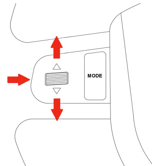
You can scroll in the Polar FIS configuration menú turning the Wheel up/down.
