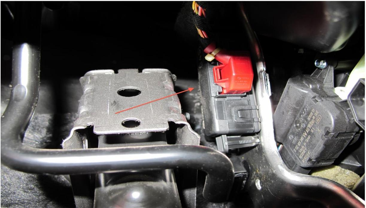
Now we must connect the Gateway connection to PolarFIS, and after then, PolarFIS to the Gateway of the car, therefore to make a “bridge”. The way in which we connect it is not important since the application works in both senses. A white connector will be free, that is not important since it is for future updates.
