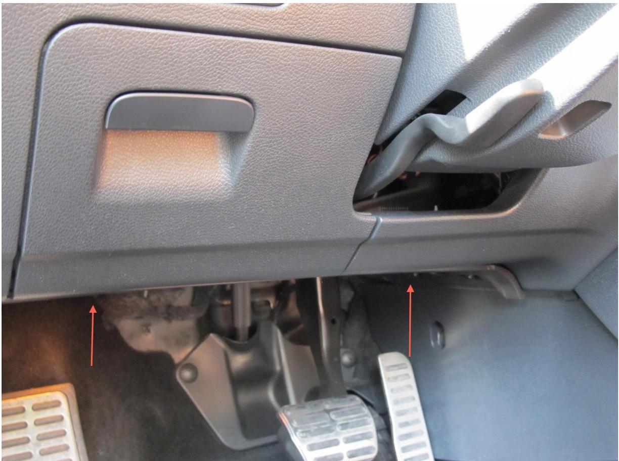
This cover has two Torx screws, and it falls throwing towards underneath.
