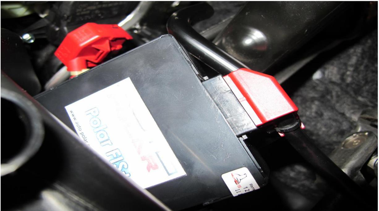
As you can see in the photography, PolarFIS has 2 connectors, you must connect the connector which you just extract from the Gateway in one of the free PolarFIS connectors (either of them is valid), next, you must connect one of the ends of the cable to the connector that is free in your PolarFIS and the other end must be connected to the Gateway.
