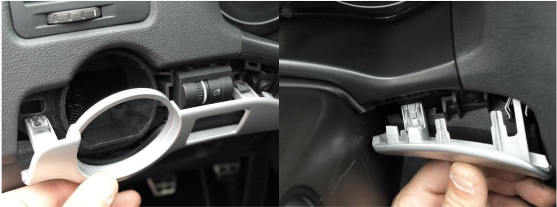
To continue, disassemble the cover of fuses compartment, introducing a blade screwdriver in order to lever, in the place indicated in the following image.
